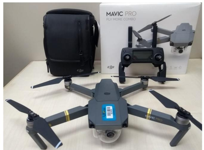
**Figure 1.** Dà-Jiàng Innovations Science and Technology (DJI) Mavic Pro quadcopter Remotely Piloted Aircraft System (RPAS)
