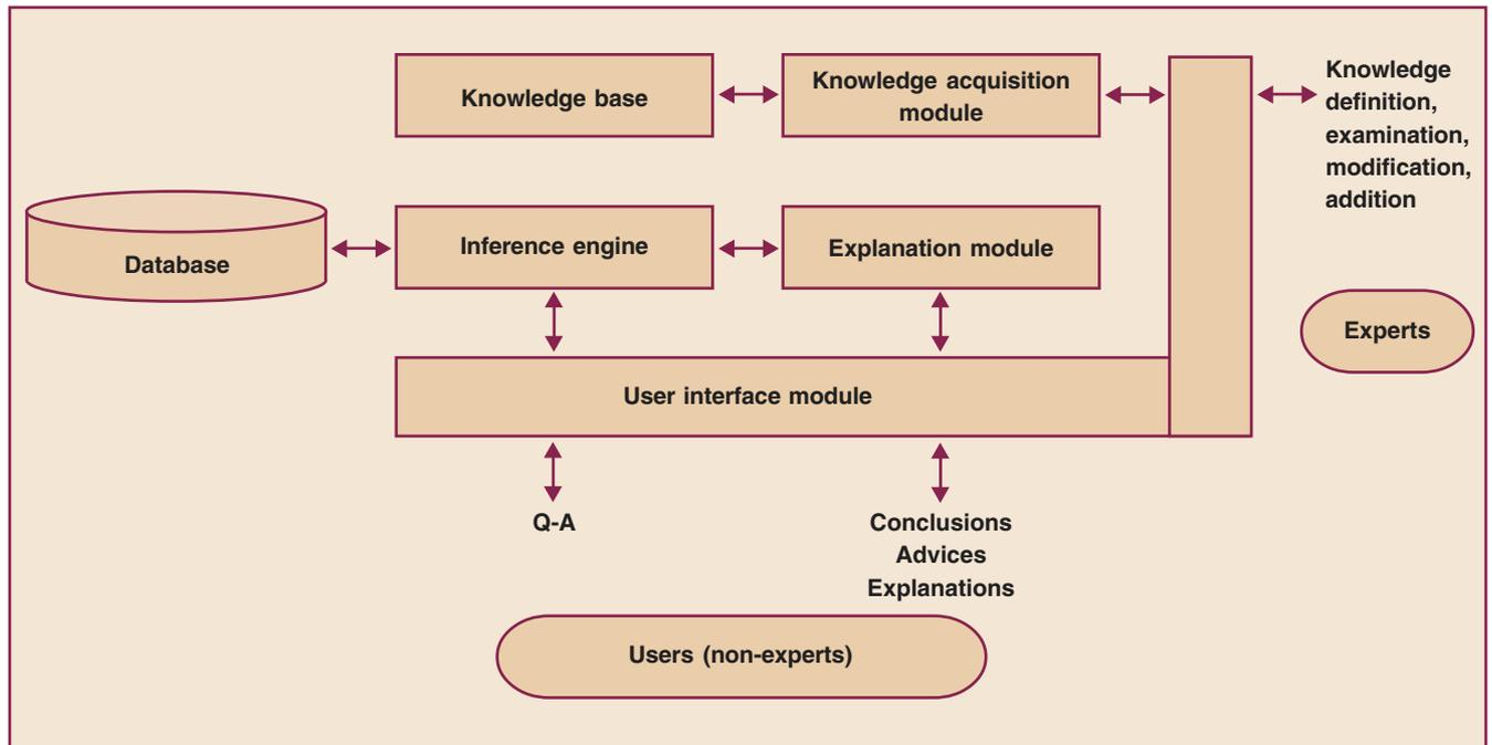
Figure 3 – A schematic representation of expert systems applied to condition-based maintenance
