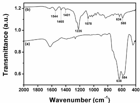
Figure 4. FTIR spectrum of (a)  $\text{Fe}_3\text{O}_4$ -NPs and (b)  $\text{Fe}_3\text{O}_4$ -NPs/PPy.
