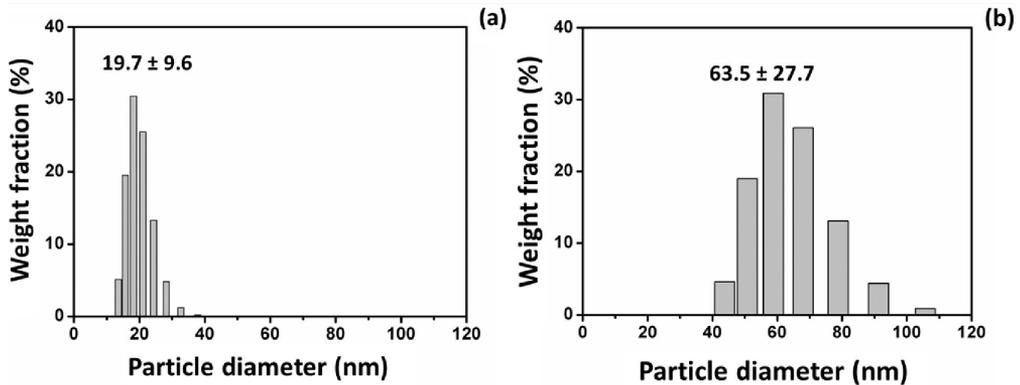
Figure 1. Size distribution of colloidal suspension particles: (a) Fe<sub>3</sub>O<sub>4</sub> NPs and (b) Fe<sub>3</sub>O<sub>4</sub> NPs/PPy characterized by DLS.
