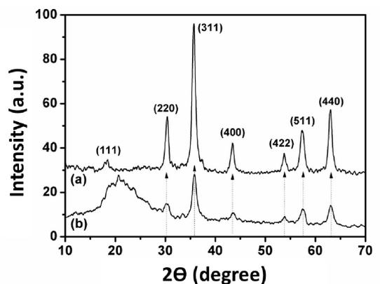
Figure 3. X-ray diffraction patterns of (a) Fe<sub>3</sub>O<sub>4</sub> NPs and (b) Fe<sub>3</sub>O<sub>4</sub> NPs/PPy.
