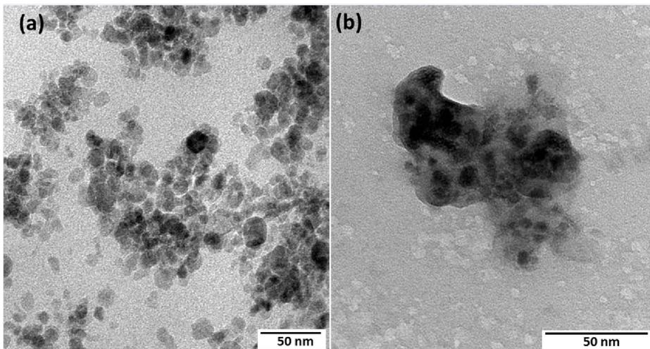
Figure 2. Images obtained by TEM of: (a) Fe<sub>3</sub>O<sub>4</sub> NPs and (b) Fe<sub>3</sub>O<sub>4</sub> NPs/PPy.
