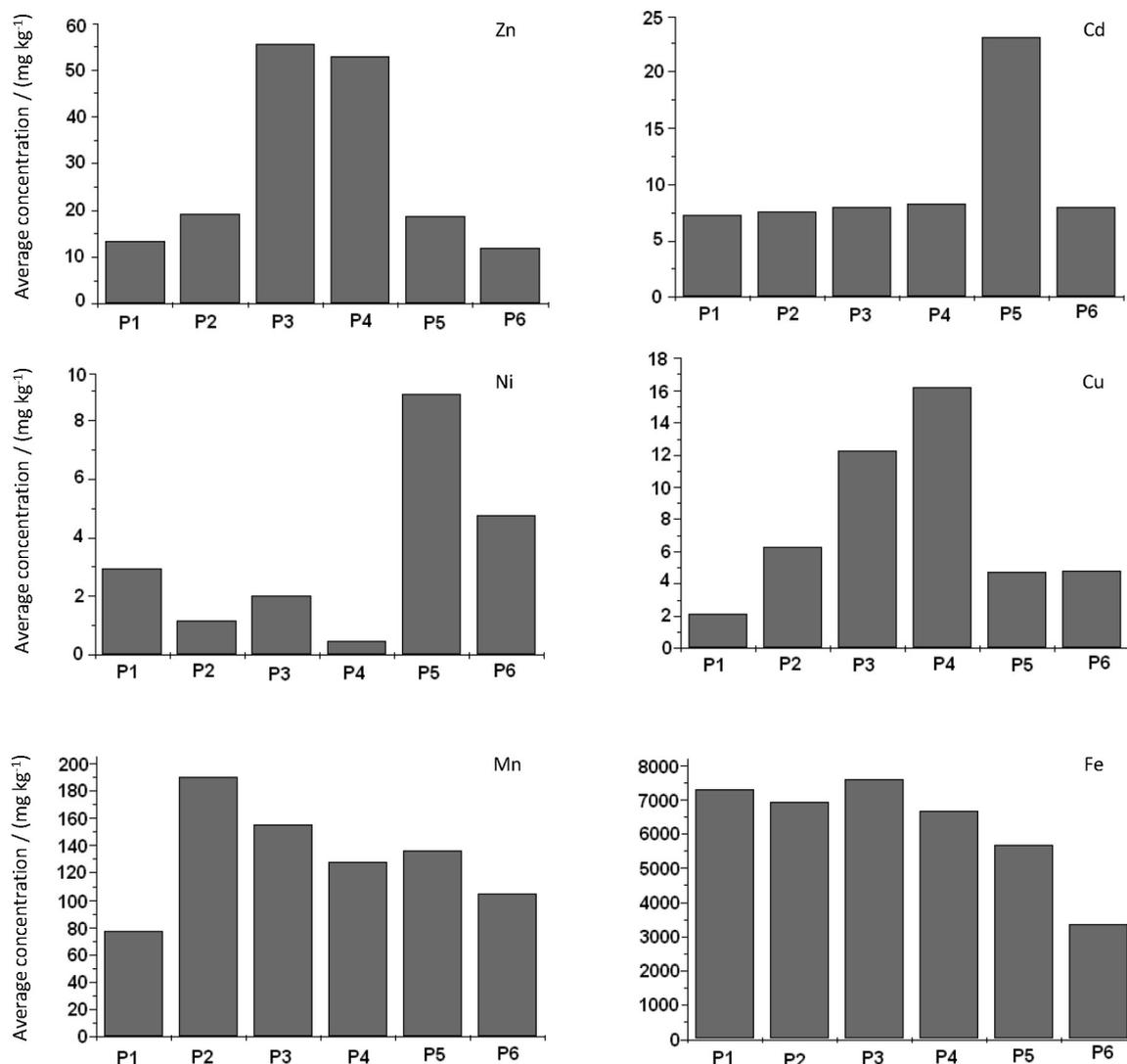
Figure 2. Average concentrations of Zn, Cd, Ni, Cu, Mn and Fe in the residual fractions of the sediments.
