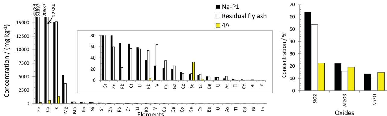
**Figure 5.** Average concentrations recorded for majority, minority and trace elements in solid products obtained by process B, obtained by XRF (majority and minority elements) and ICP-MS (trace elements).
