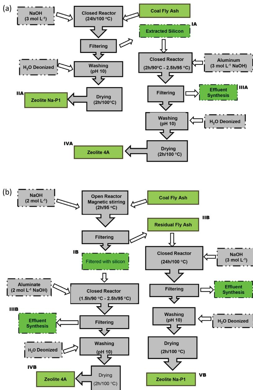
**Figure 1.** Flow diagrams of integrated zeolite synthesis via (a) process A and (b) process B. Rectangles depict material input and output in the solid (solid line) and aqueous (dashed line) steps, while rectangles with arrows indicate operations. Roman numerals indicate outputs for which the chemical composition was measured.
