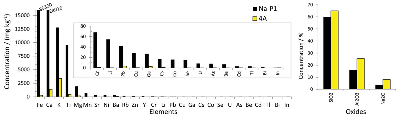
**Figure 3.** Average concentrations obtained for the majority, minority and trace elements in synthetic zeolites using process A. Results obtained by XRF (majority and minority elements) and ICP-MS (trace elements).
