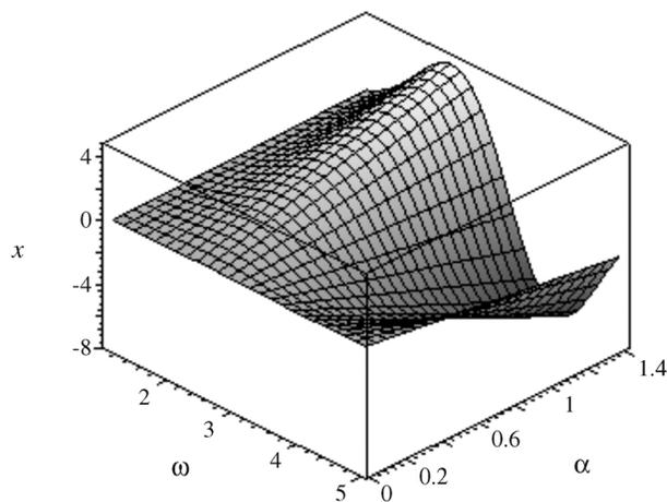
**Figure 4** - The surface  $\chi(\omega, \alpha)$  - volume of a tetrahedron unit cell - the chirality constraint.
