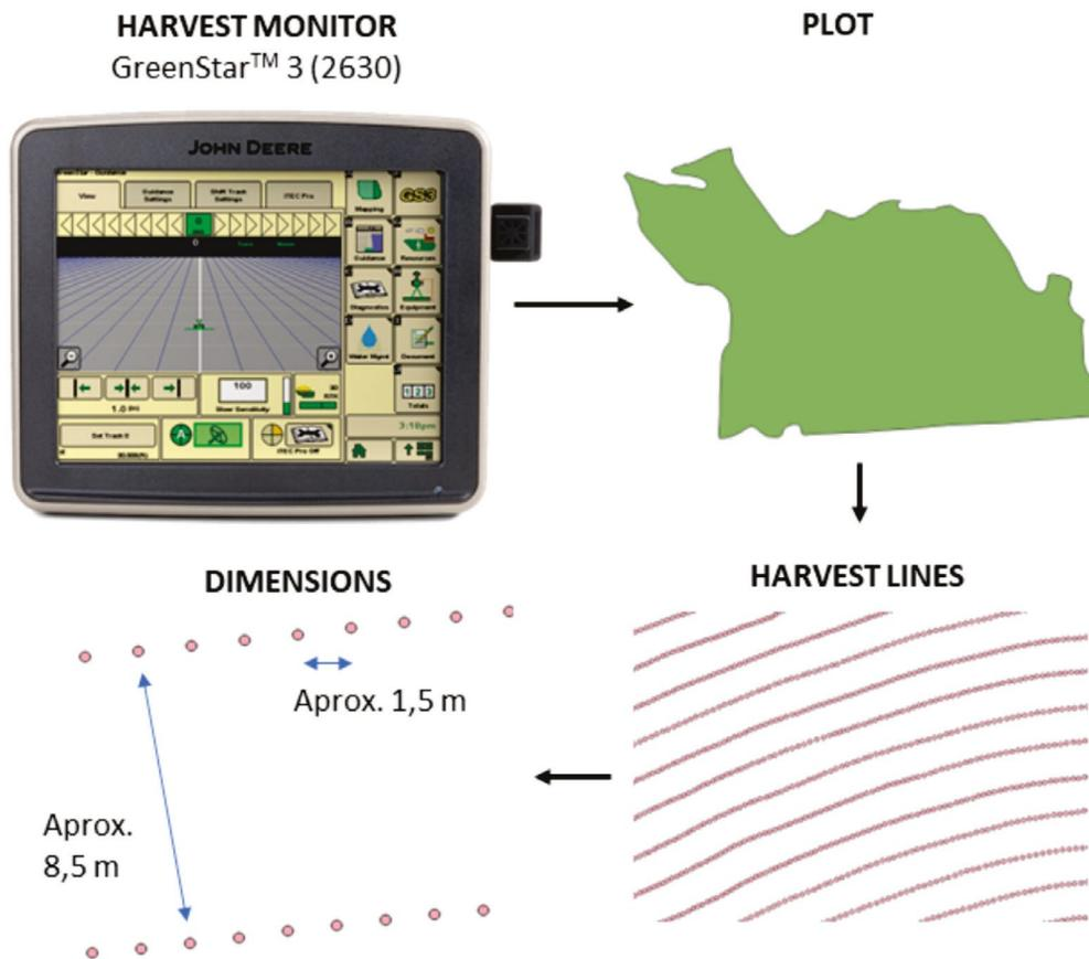
**Figure 2:** General scheme for obtaining soybean harvest data in plots. Adapted from John Deere (2022).
