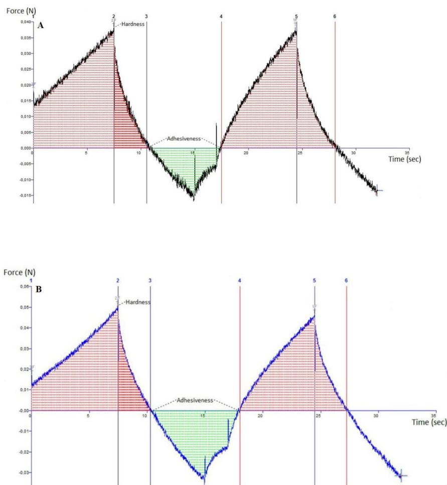
**FIGURE 4** - Texture profile analysis graphs of hydrogel formulations (a: A2, b: F2). All of the formulations have texture profile analysis graphs but A2 and F2 formulations were selected because these formulations were optimized in terms of mechanical properties. The first peak of the graphs expresses the hardness value. The area under the curve between 3 and 4 (AUC3-4) is calculated as the adhesion value.
