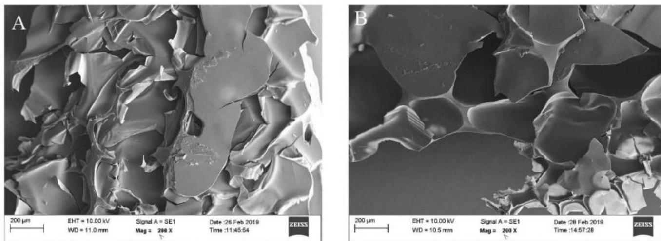
**FIGURE 1** - Scanning electron photomicrographs of chitosan-PVA hydrogel surface morphology (A: B1 formulation, B: F2 formulation).
