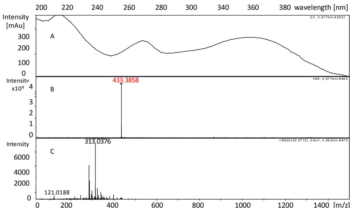
**FIGURE 1** - UV-UHPLC (A) /EIC MS (B) /Fragmentation pattern (C) of F4.3.2 (M+H)<sup>+</sup> 433.3858 Da, retention time, tR 4.977 min.
