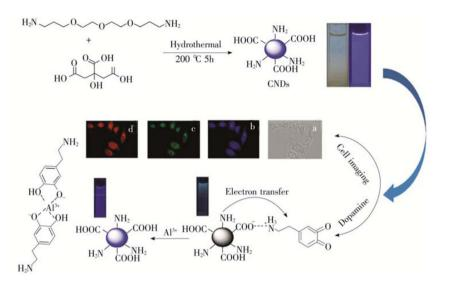
Figure 3. Carbon dots are synthesized and used as a fluorescent probe for Al<sup>3+</sup>.
