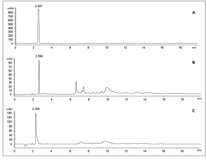
**FIGURE 1** - Chromatographic profile of the 5-CQA standard (A), CP01/5-CQA coelution (B) and CP02/5-CQA coelution (C) by HPLC-UV. The detection wavelength was at 330 nm. CP01: glycerin (GLY - 70 %) and grain alcohol (GA - 30 %); CP02: propylene glycol (PG - 70 %) and grain alcohol (GA - 30 %); 5-CQA: 5-O-caffeoylquinic acid.
