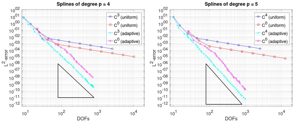
Figure 5: The decay of  $\|g - \mathcal{Q}_1(g)\|_{L^2}$  for splines of degrees 4 (left) and 5 (right) with maximum smoothness and globally continuous splines of the same degrees onto uniform and adaptive meshes.
