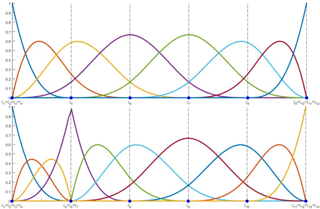
Figure 1: Examples of cubic B-splines of maximum smoothness (top) and with a triple internal knot (bottom).
