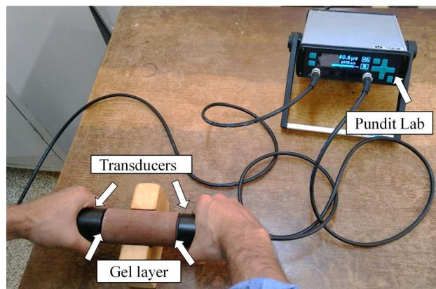
Figure 2. Ultrasonic test execution.
