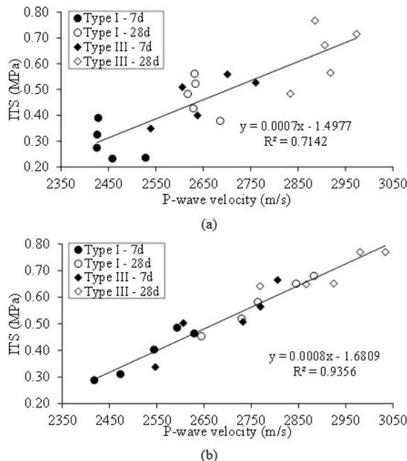
**Figure 8.** Relation between P-wave velocity and ITS for: (a) CD and (b) RD.
