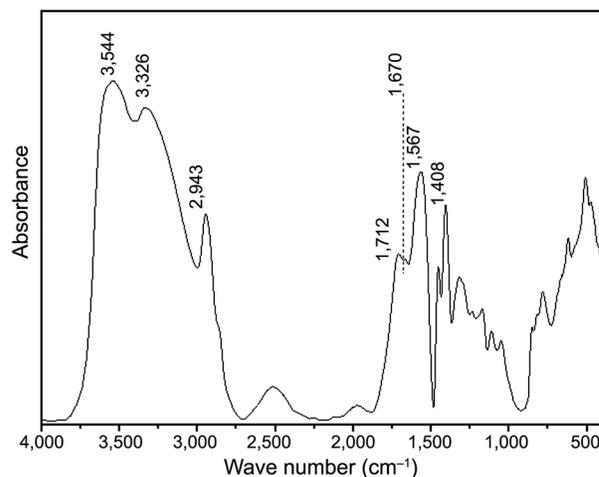
**Figure 1** – Fourier Transform Infrared Spectroscopy (FTIR) spectra of hydrogel powder in potassium bromide (KBr) pellet.
