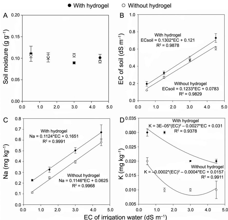
**Figure 5** – Attributes evaluated in the soil in response to both irrigation water EC ( $\text{dS m}^{-1}$ ) and hydrogel treatments (with and without). (A) Soil moisture at the end of experimental period ( $\text{g g}^{-1}$ ); (B) Soil solution EC ( $\text{dS m}^{-1}$ ); (C) Exchangeable soil  $\text{Na}^+$  content ( $\text{mg kg}^{-1}$ ); and (D) Exchangeable soil  $\text{K}^+$  content ( $\text{mg kg}^{-1}$ ).
