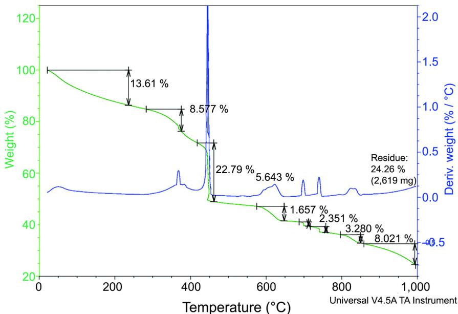
**Figure 2** – Thermal Gravimetric Analysis (TGA) and its first derivative (DTG) curves of hydrogel in air atmosphere.
