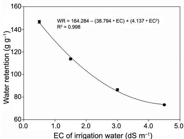
**Figure 3** – Water retention by hydrogel (g g<sup>-1</sup>) in response to increasing electrical conductivity (EC in dS m<sup>-1</sup>) of irrigation water in laboratory.
