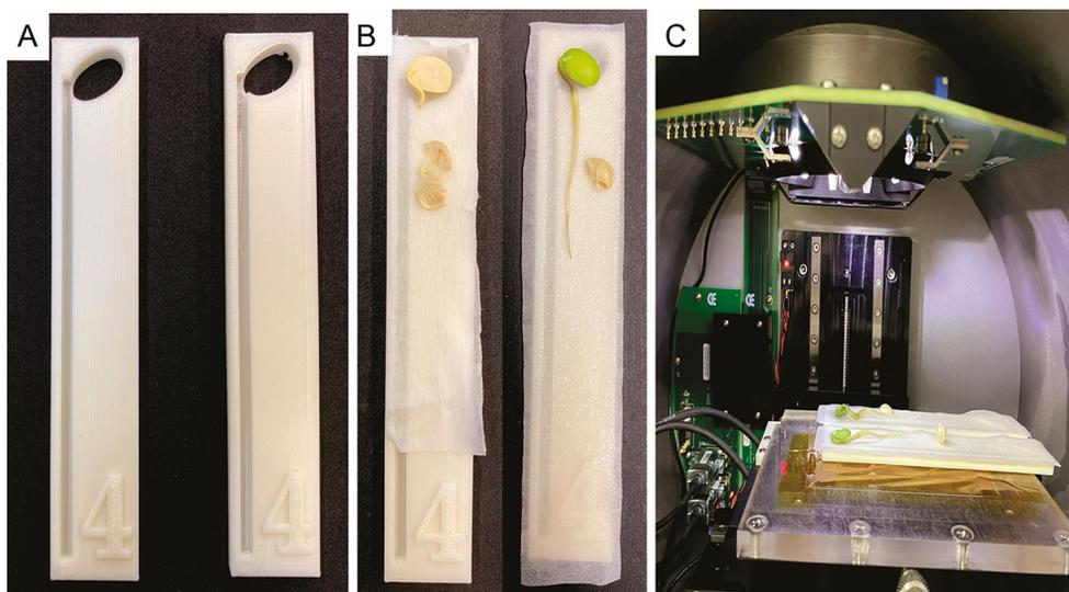
**Figure 2** – Sample holder for seedling analysis (A), positioning of seedlings on the sample holder (B) and positioning of the sample holder in the equipment (C). Source: Rohr (2021).
