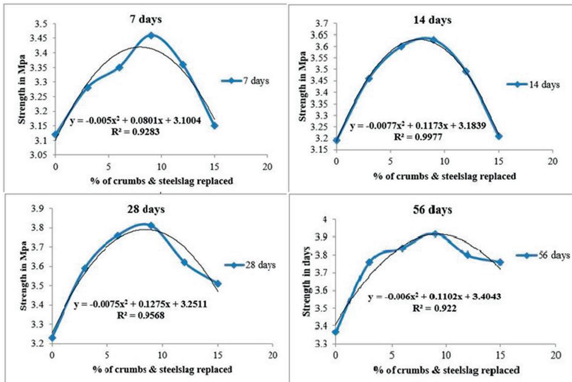
**Figure 7:** a) A trend of split tensile strength vs. % of rubber crumbs + steel slag for 7 days curing spell, b) A trend of split tensile strength vs. % of rubber crumbs + steel slag for 14 days curing spell, c) A trend of split tensile strength vs. % of rubber crumbs + steel slag for 28 days curing spell, d) A trend of split tensile strength vs. % of rubber crumbs + steel slag for 56 days curing spell.
