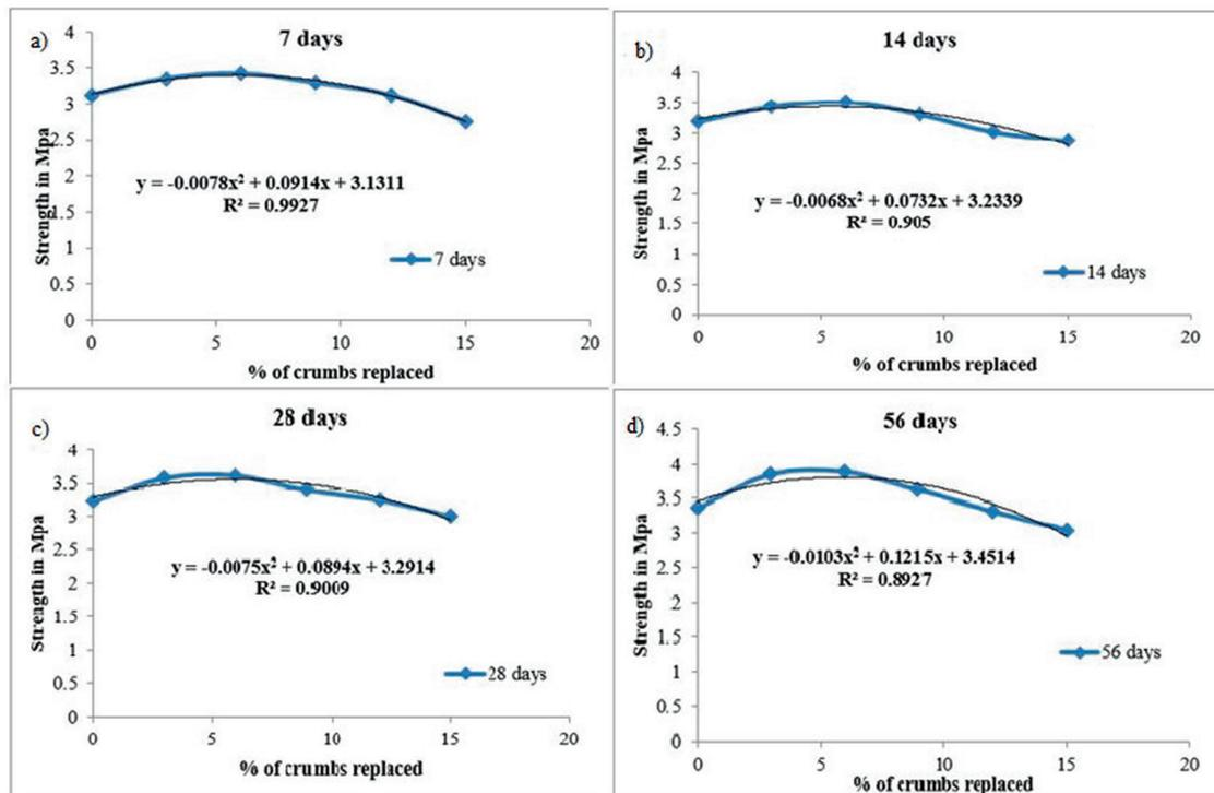
**Figure 5:** a) A trend of split tensile strength vs. % of rubber crumbs for 7 days curing spell, b) A trend of split tensile strength vs. % of rubber crumbs for 14 days curing spell, c) A trend of split tensile strength vs. % of rubber crumbs for 28 days curing spell, d) A trend of split tensile strength vs. % of rubber crumbs for 56 days curing spell.
