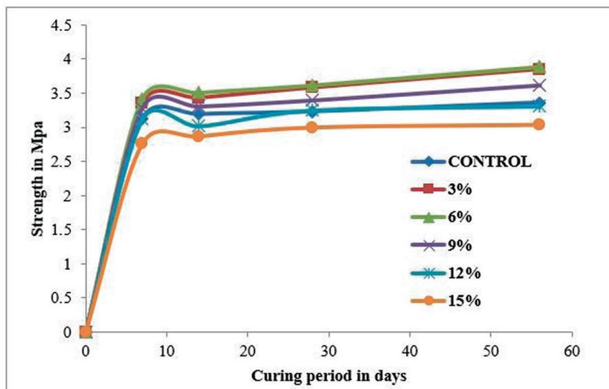
Figure 2: A family of curves (rubber crumbs against fine aggregate) for split tensile strength vs. curing spell in days.
