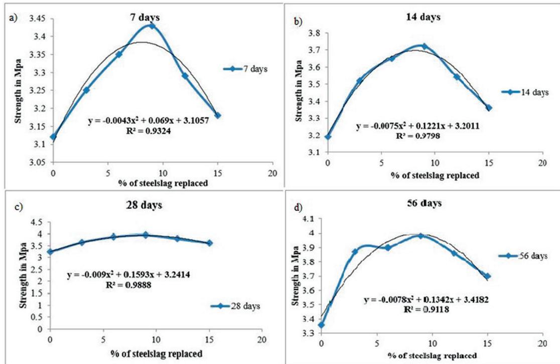
**Figure 6:** a) A trend of split tensile strength vs. % of steel slag for 7 days curing spell b) A trend of split tensile strength vs. % of steel slag for 14 days curing spell, c) A trend of split tensile strength vs. % of steel slag for 28 days curing spell, d) A trend of split tensile strength vs. % of steel slag for 56 days curing spell.
