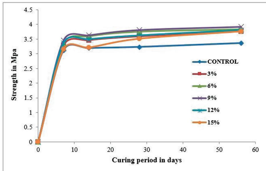
**Figure 4:** A family of curves (rubber crumbs + steel slag against fine aggregate and cement) for split tensile strength vs. curing spell in days.
