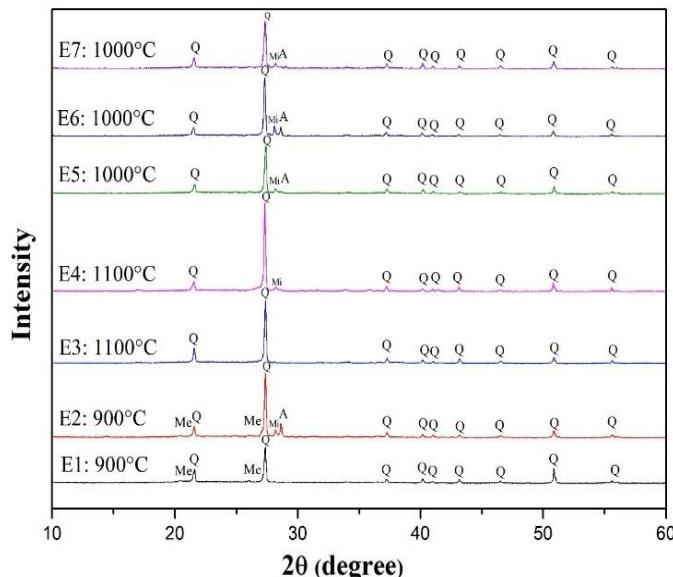
**Figure 2:** X-ray diffractogram of the Sintered Essays: Q - quartz, Me - metakaolinite, Mi - microcline and A - albite.
