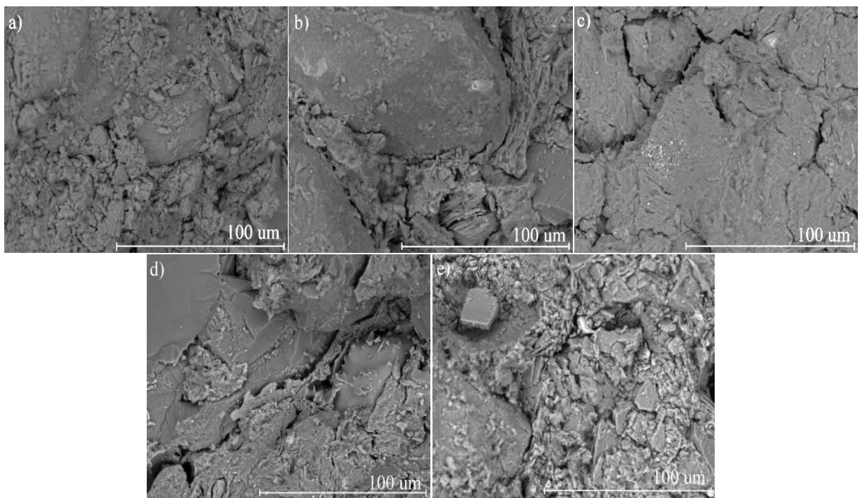
**Figure 3:** Scanning electron microscopy images of sintered formulations. (a) 0% of granite waste sintered at 1173K; (b) 20% of granite waste sintered at 1173K; (c) 0% of granite waste sintered at 1373K; (d) 20% granite waste sintered at 1373K; (e) 10% granite waste sintered at 1273K.
