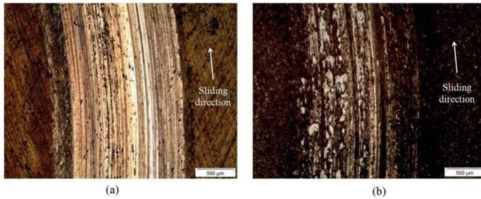
**Figure 7:** Optical micrography of the wear track (1928 m travelled): (a) Non-shot peened specimen (b) Shot peened specimen.
