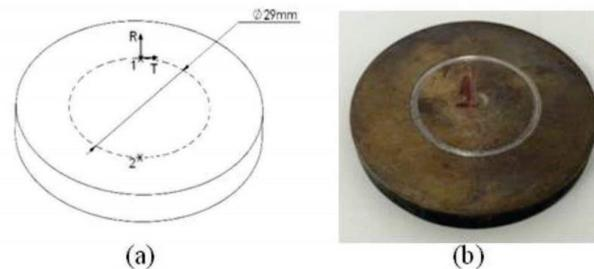
**Figure 1:** AISI 4340 disks used in wear tests: (a) Dimensions; (b) Worn surface.
