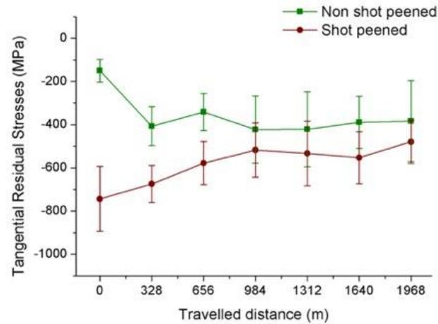
Figure 5: Tangential residual stresses during pin-on-disk test.
