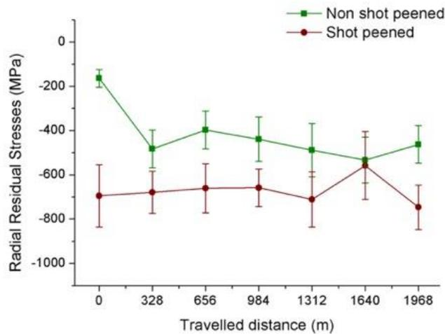
Figure 6: Radial residual stresses during pin-on-disk test.
