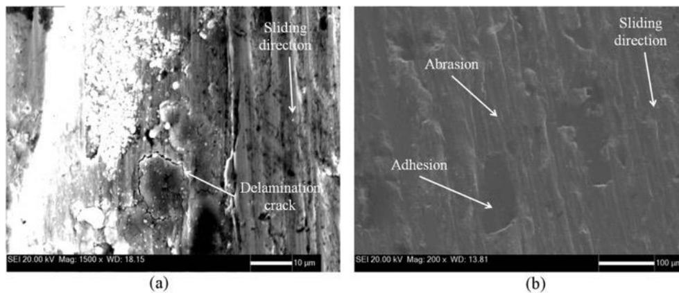
**Figure 8:** SEM micrography of wear track (1928 m travelled): (a) Non-shot peened specimen (b) Shot peened specimen.
