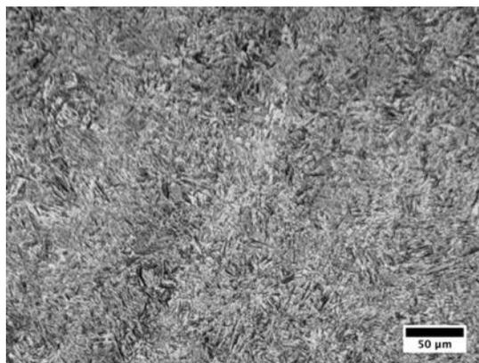
**Figure 2:** Tempered martensite microstructure. Optical microscopy.
