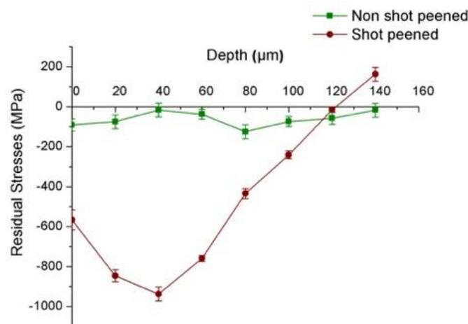
**Figure 4:** Depth residual stress profile before wear tests.
