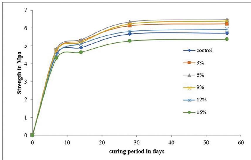
Figure 5: A family of curves (rubber crumbs and coal ash against fine aggregate and cement) for flexural strength Vs. curing spell in days.
