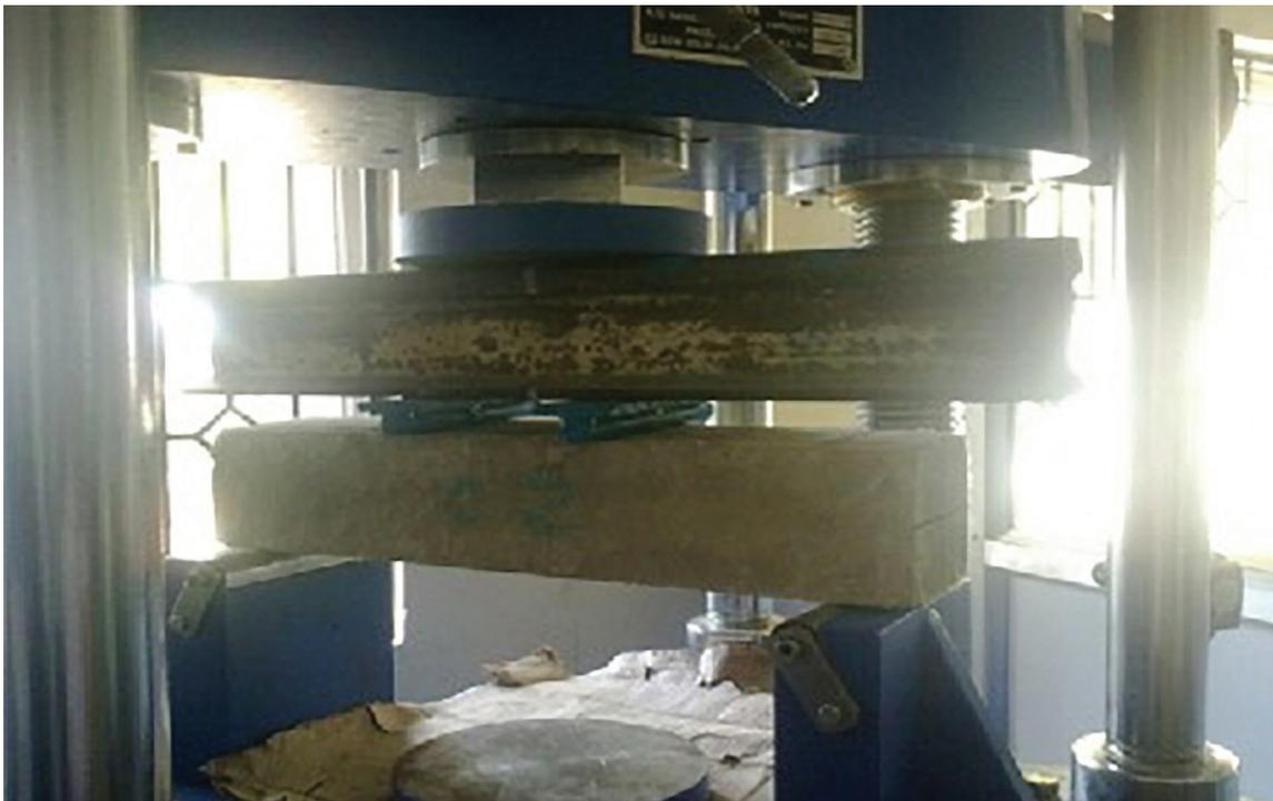
**Figure 1:** Flexural strength test setup.
