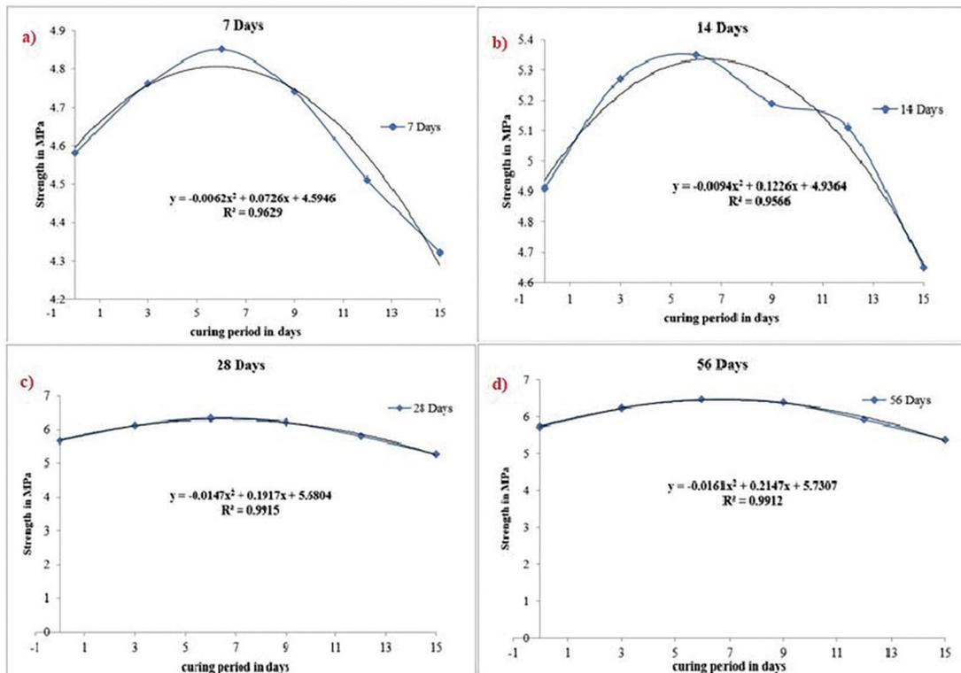
Figure 8: (a) A trend of flexural strength Vs. % of rubber crumbs and coal ash for 7 days curing spell, (b) A trend of flexural strength Vs. % of rubber crumbs and coal ash for 14 days curing spell, (c) A trend of flexural strength Vs. % of rubber crumbs and coal ash for 28 days curing spell, (d) A trend of flexural strength Vs. % of rubber crumbs and coal ash for 56 days curing spell.
