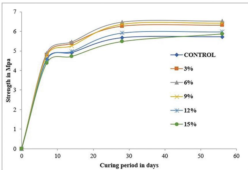
Figure 4: A family of curves (coal ash against cement) for flexural strength Vs. curing spell in days.
