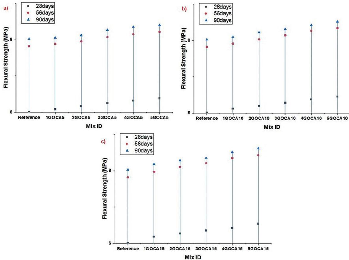
Figure 2: Flexural strength of Coal ash (5% to 15%) concrete with graphene oxide (0.1% to 0.5%).
