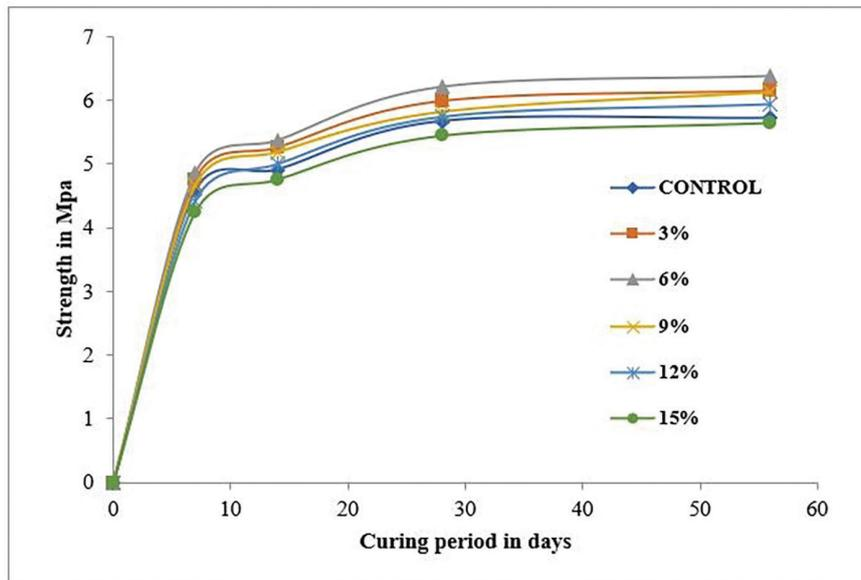
Figure 3: A family of curves (rubber crumbs against fine aggregate) for flexural strength Vs. curing spell in days.
