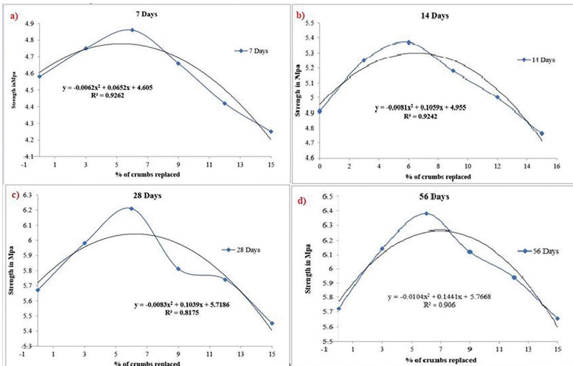
Figure 6: (a) A trend of flexural strength Vs. % of rubber crumbs for 7 days curing spell, (b) A trend of flexural strength Vs. % of rubber crumbs for 14 days curing spell, (c) A trend of flexural strength Vs. % of rubber crumbs for 28 days curing spell, (d) A trend of flexural strength Vs. % of rubber crumbs for 56 days curing spell.
