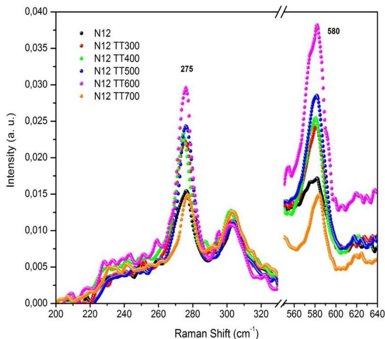
Figure 5: Raman spectra of N12 sample after thermal treatment at different temperatures, compared with the spectrum without treatment.
