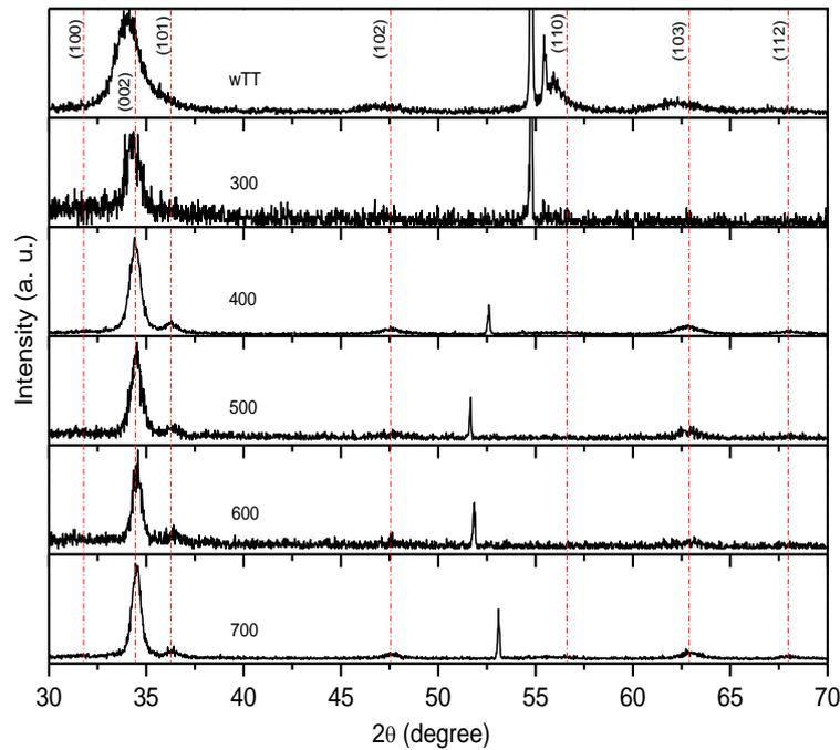
Figure 4: XRD patterns of N12 after thermal treatment compared with the spectra without thermal treatment (wTT).
