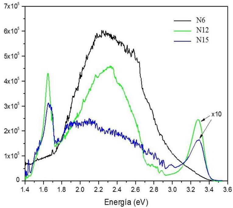
**Figure 2:** Room temperature photoluminescence of Al-N codoped ZnO with 6, 12 and 15 sccm nitrogen flow. The N12 and N15 spectra were magnified by 10.
