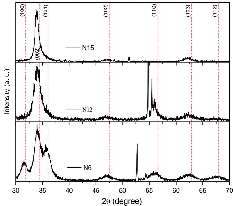
**Figure 1.** XRD patterns of ZnO films as-growth with flow rate nitrogen of 6 (N6), 12 (N12) and 15 sccm (N15) before thermal treatment. Red lines indicate location peak for undoped ZnO films.
