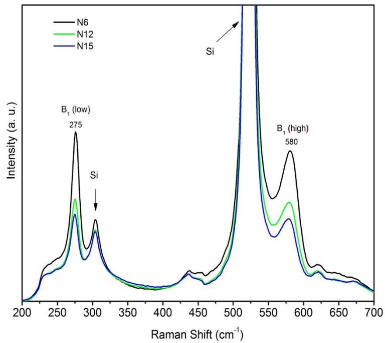
**Figure 3:** Raman spectra of ZnO films codoped with 6 (N7), 12 (N12) and 15 sccm (N15) nitrogen flow.
