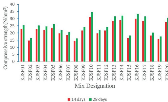
Figure 2: Compressive strength of fibre reinforced concrete.
