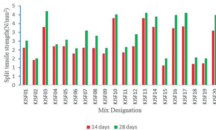
Figure 3: Split tensile strength of fibre reinforced concrete.
