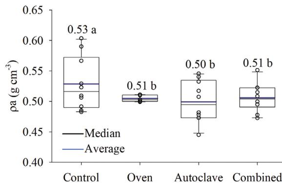
**Figure 2:** Values of apparent density ( $\rho a$ ) for the GG100 clone wood before (control) and after different thermal treatments (T1, T2, and T3).
