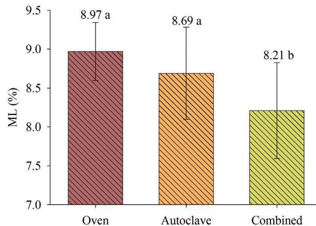
**Figure 3:** Mass loss (ML) of the GG100 clone wood before (control) and after different thermal treatments (T1, T2, and T3). \*Values above the bars indicate that means followed by the same letters do not differ from each other by the Scott-Knott test at 95% probability.
