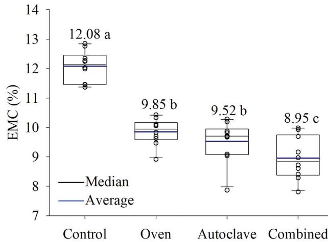
**Figure 4:** Equilibrium moisture values (EMC) for the GG100 clone wood before (control) and after different heat treatments T1, T2, and T3.
