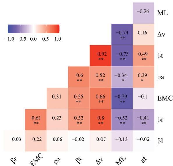
**Figure 6:** Correlogram from the Pearson correlation analysis of the physical properties, as follows: apparent density ( $\rho_a$ ); mass loss (ML); longitudinal ( $\beta_l$ ), radial ( $\beta_r$ ), tangential ( $\beta_t$ ), and volumetric ( $\Delta v$ ) shrinkages; anisotropy factor ( $\alpha_f$ ); and equilibrium moisture content (EMC) obtained for the GG100 clone wood after different heat treatments.
