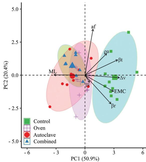
**Figure 5:** Perceptual map with the results of the principal component analysis (PCA) for apparent density ( $\rho_a$ ); mass loss (ML); longitudinal ( $\beta_l$ ), radial ( $\beta_r$ ), tangential ( $\beta_t$ ), and volumetric ( $\Delta_v$ ) shrinkages; anisotropy (fa); and equilibrium moisture content (EMC); and grouping of physical properties before (control) and after treatments (T1, T2, and T3) applied to GG100 clone wood.
