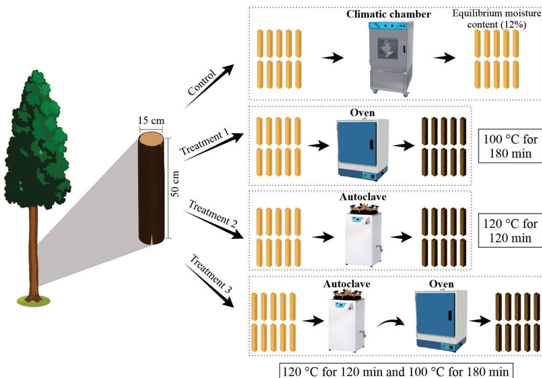
Figure 1: General scheme of thermal treatments applied to the GG100 clone.
