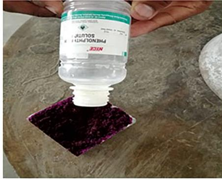
Figure 15: Carbonation Test.
