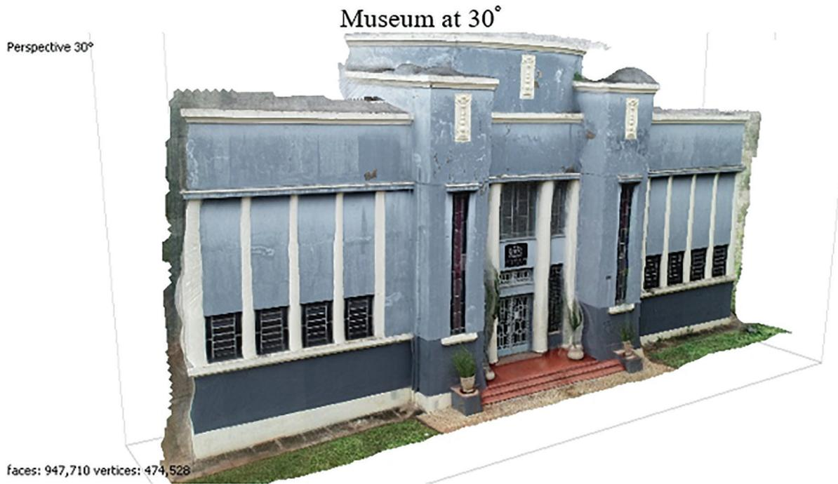
**Figure 10:** Photogrammetric model of the main façade of the Zoroastro Artiaga.
