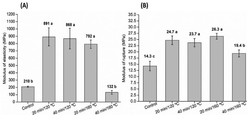
**Figure 6:** (A) Modulus of elasticity (MOE); and (B) modulus of rupture of the hardboards subjected to flexural strength (Tukey test,  $p > 0.05$ ).
