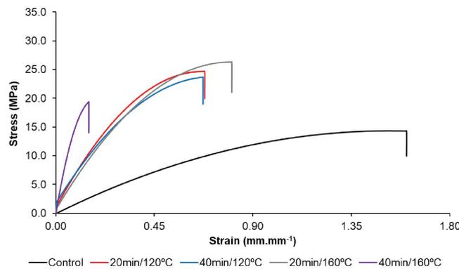
**Figure 7:** Stress × strain curves for the bending test of the different evaluated treatments.
