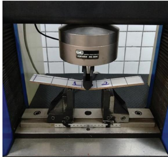
Figure 2: Flexural strength test in three points.
