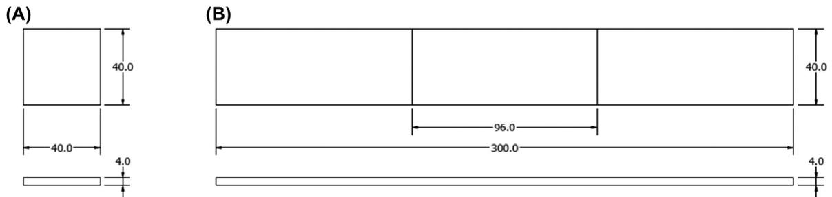
**Figure 1:** Samples for physical and mechanical tests (dimensions in mm); (A) physical tests: bulk density, moisture content, water absorption, thickness swelling, and non-return rate in thickness; (B) flexural strength (three points).
