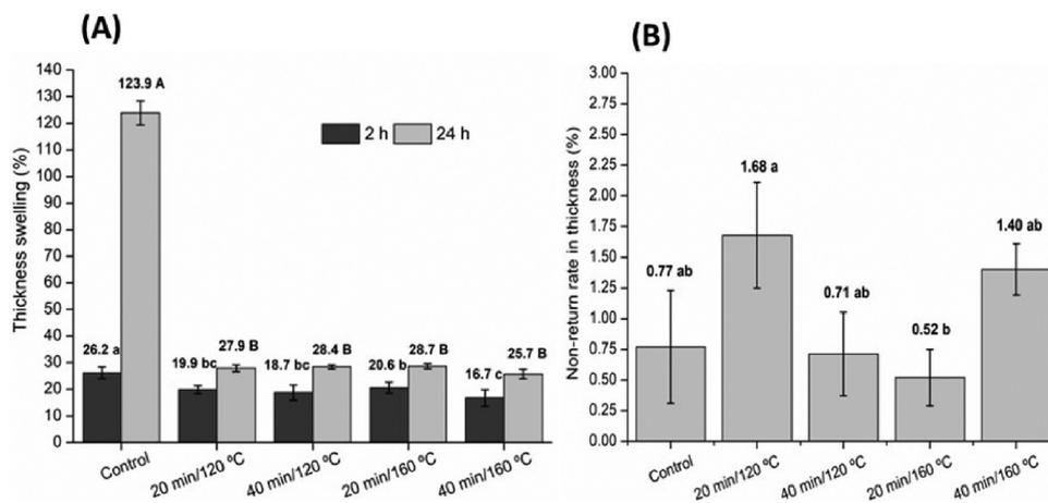
**Figure 5:** (A) Thickness swelling at 2 and 24 h; and (B) non-return rate in thickness; averages followed by the same uppercase or lowercase letter do not differ (Tukey test,  $p > 0.05$ ).
