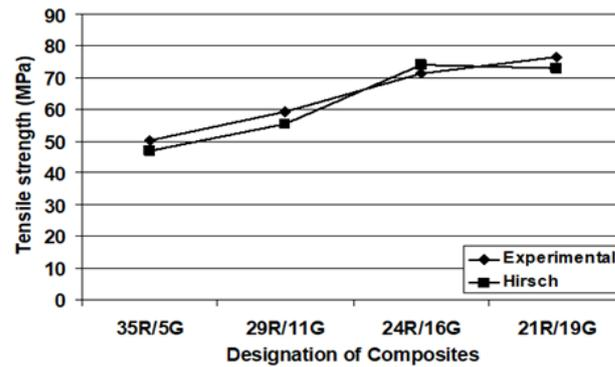
**Figure 9:** Predicted and experimental results of tensile strength in the Skin-core type composites
