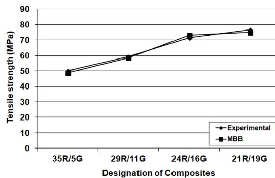
**Figure 10:** Predicted and experimental results of tensile strength in the Skin-core type composites
