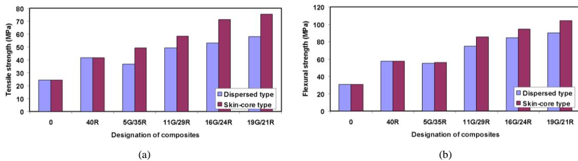
**Figure 8:** Comparison of (a) tensile strength and (b) flexural strength values of dispersed and skin-core type composites
