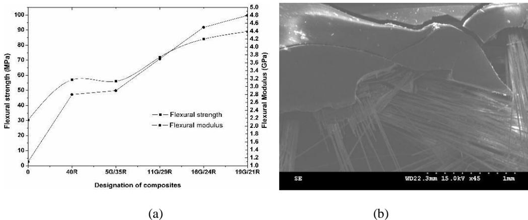
**Figure 6:** (a) Variation of flexural strength and modulus, (b) SEM image of the fracture surface of 21R/19G composites (dispersed type) after the flexural test
