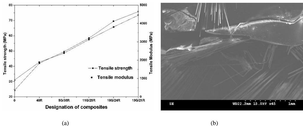
**Figure 5:** (a) Variation of tensile strength and modulus, (b) SEM image of fracture surface of 21R/19G composites (skin-core type) after tensile test.
