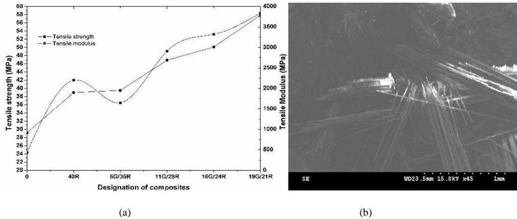
**Figure 4:** (a) Variation of tensile strength and modulus, (b) SEM image of the fracture surface of 21R/19G composites (dispersed type) after the tensile test
