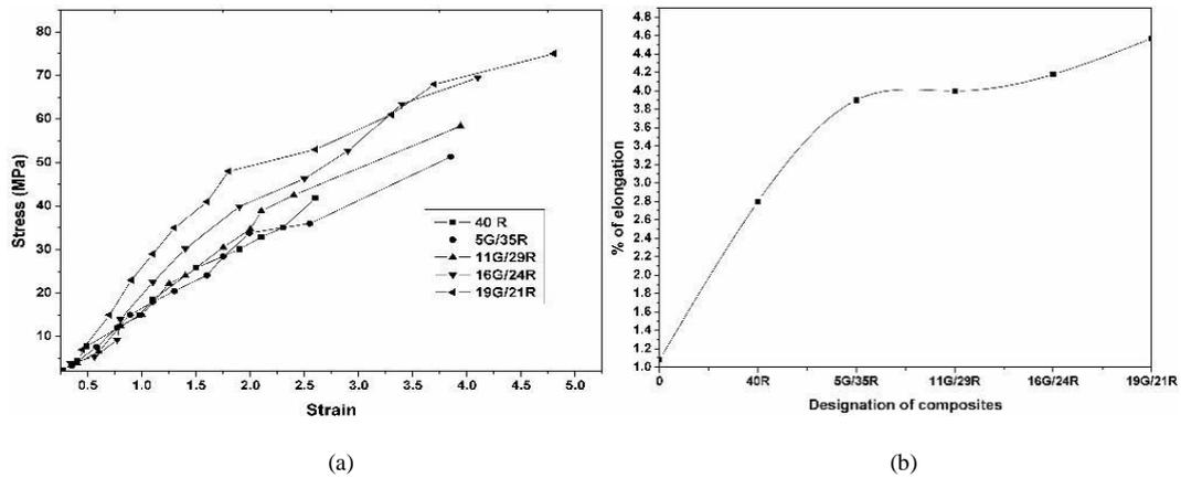
**Figure 3:** (a) Stress-strain curves and (b) variation of % of elongation of Pineapple/glass fiber hybrid composite (skin-core type)
