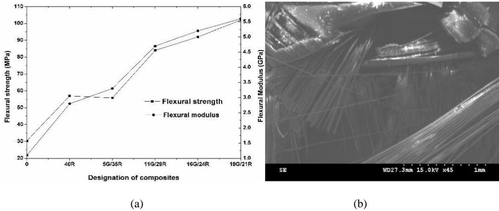
**Figure 7:** (a) Variation of flexural strength, (b) SEM image of the fracture surface of 21R/19G composites (skin-core type) after the flexural test.
