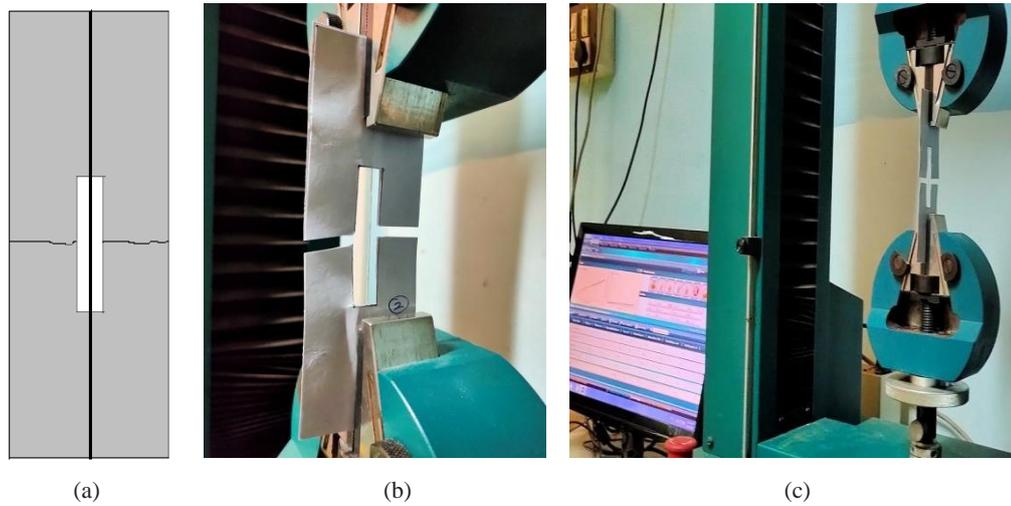
**Figure 1:** (a) Methodology of single fiber test (b), and (c) digital image of tensile fiber test at universal testing machine
