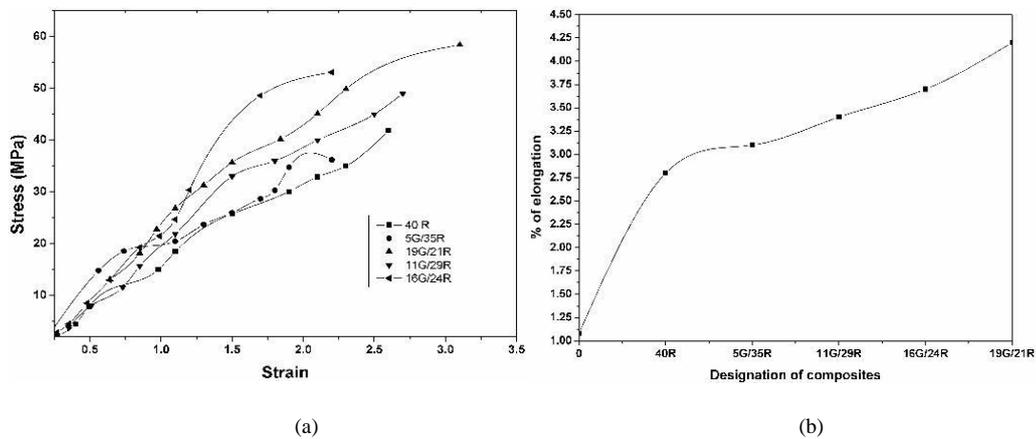
**Figure 2:** (a) Stress-strain curves and (b) variation of % of elongation of Pineapple/glass fiber hybrid composite (dispersed type)
