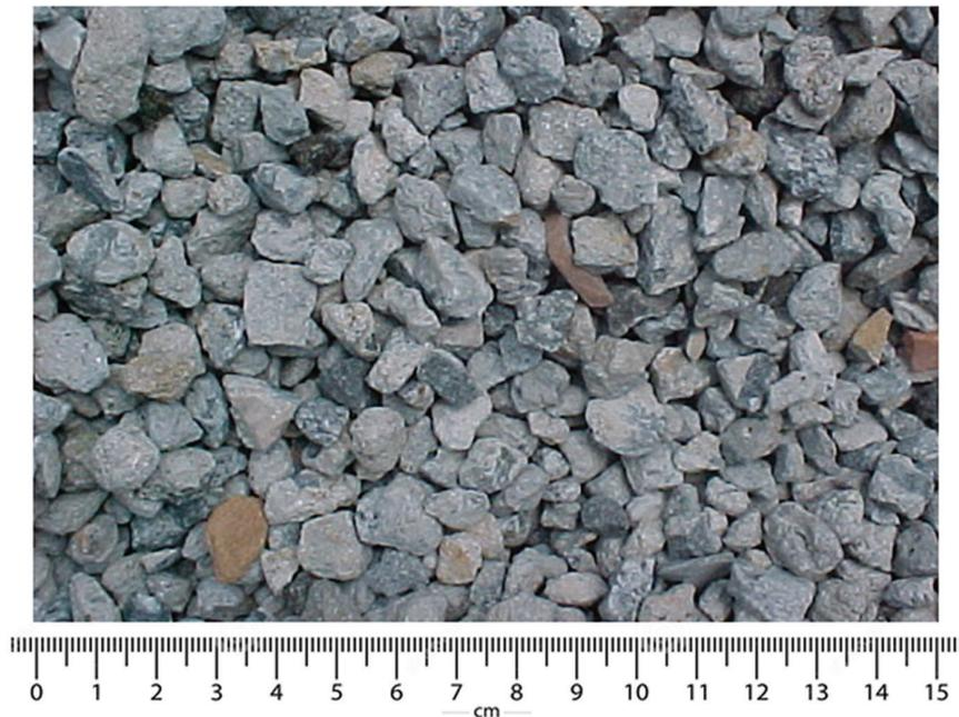
Figure 1: Coarse recycled aggregate used in the study.
