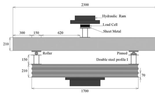
a) Characteristics and dimensions of the beams;
