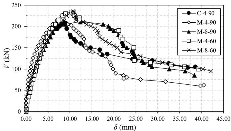
Figure 8 – Shear force versus Deflection of the beams.
