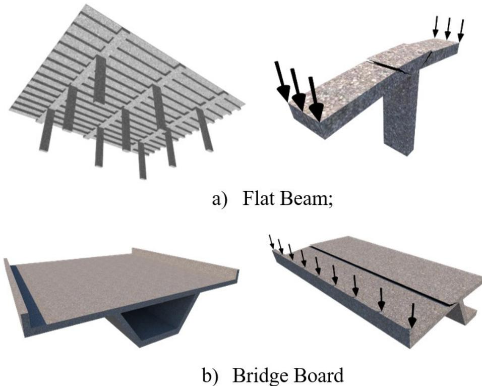
**Figure 1** - Structures under one-way shear failure.
