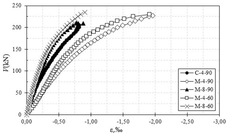
Figure 10 – Shear force versus Concrete Strain.
