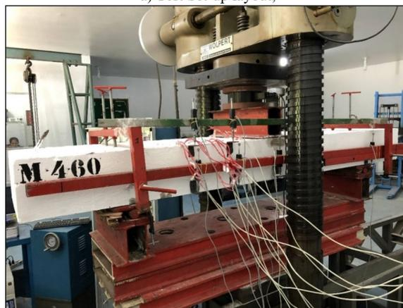
b) Beam positioned in the test set-up
