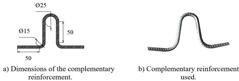
**Figure 6 – Complementary reinforcement.**
