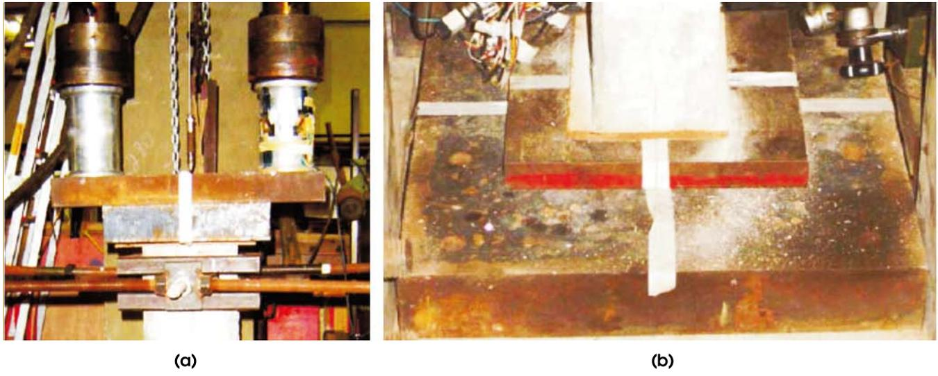
Figure 7 - Columns failure region
