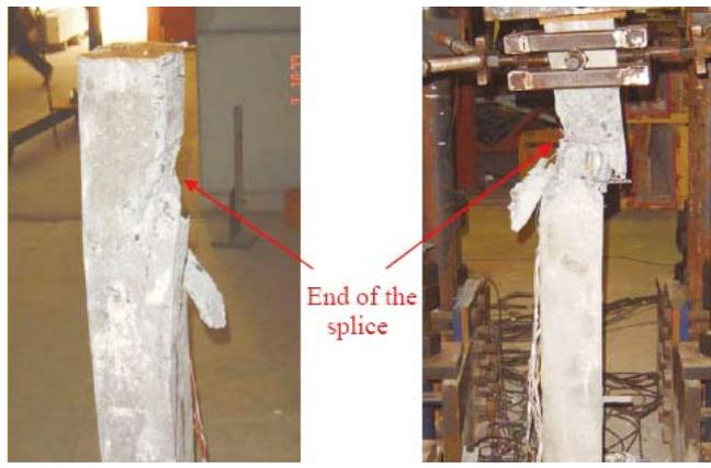
Figure 8 - Detail of the failure region
