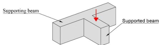
**Figure 5.** Indirect support where  $h_1 = h_2$
