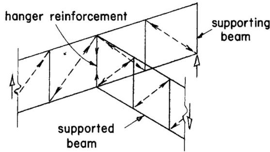
Figure 2. Strut and tie model in indirect supports [7]
