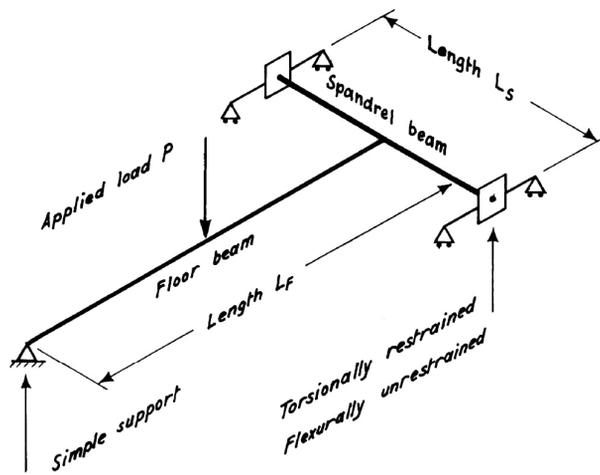
Figure 27. Structural scheme used by Collins and Lampert [9]
