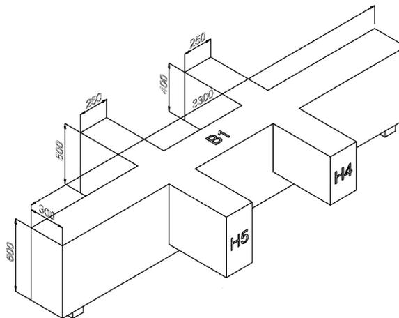
Figure 13. Description of specimen B1 (dimensions in mm) [1]
