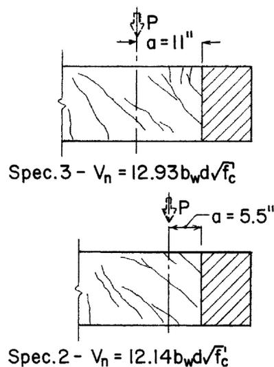
**Figure 24.** Cracking pattern of specimens 2 and 3 [7]
