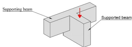
**Figure 8.** Indirect support where  $h_1 > h_2$
