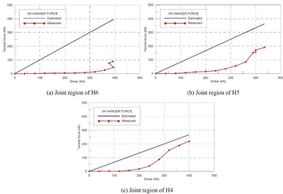
Figure 16. Tensile force on hanger reinforcement [1]
