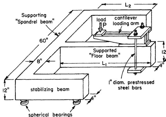
Figure 23. Typical structure of the tested specimens [7]
