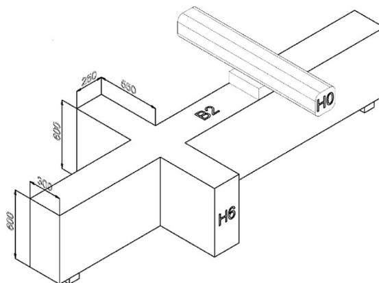
Figure 14. Description of specimen B2 (dimensions in mm) [1]
