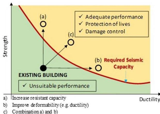
Figure 1. Earthquake-resistant capacity curve.
