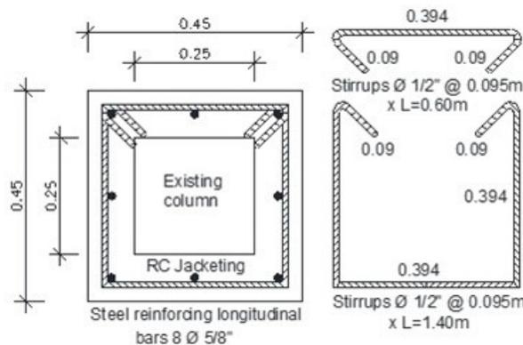
Figure 12. Column with RC Jacketing.
