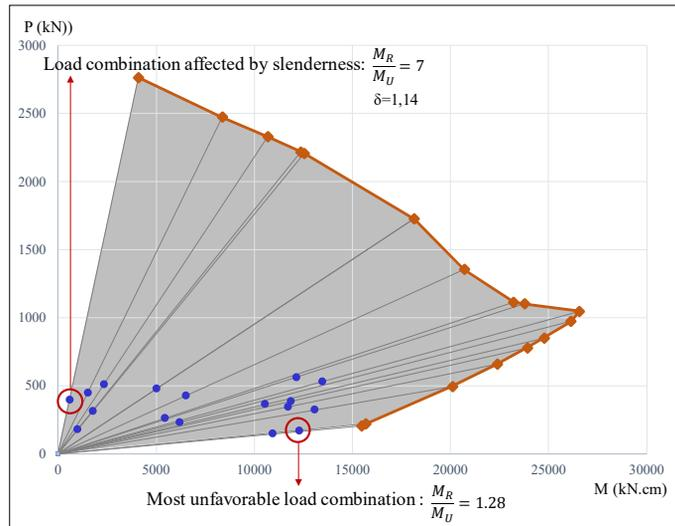
Figure 16. Interaction curve  $(P, M_y)$  for 2B column.
