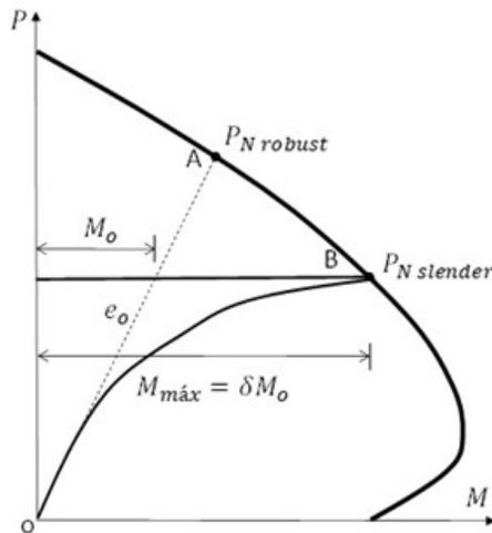
Figure 3. Effect of slenderness on carrying capacity.
