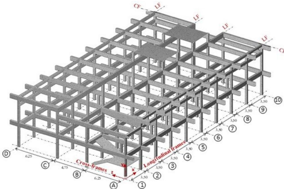
Figure 10. Building Structural System.
