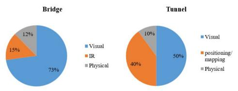
Figure 2. Percentage of the main UAV-based applications for bridge and tunnel inspection.
