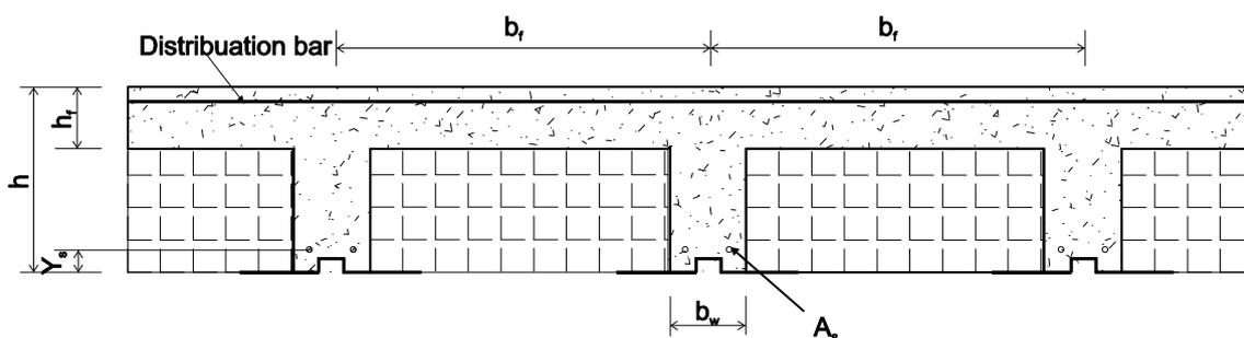
Figure 3 – Model with ceramic tile (dimensions in mm)
