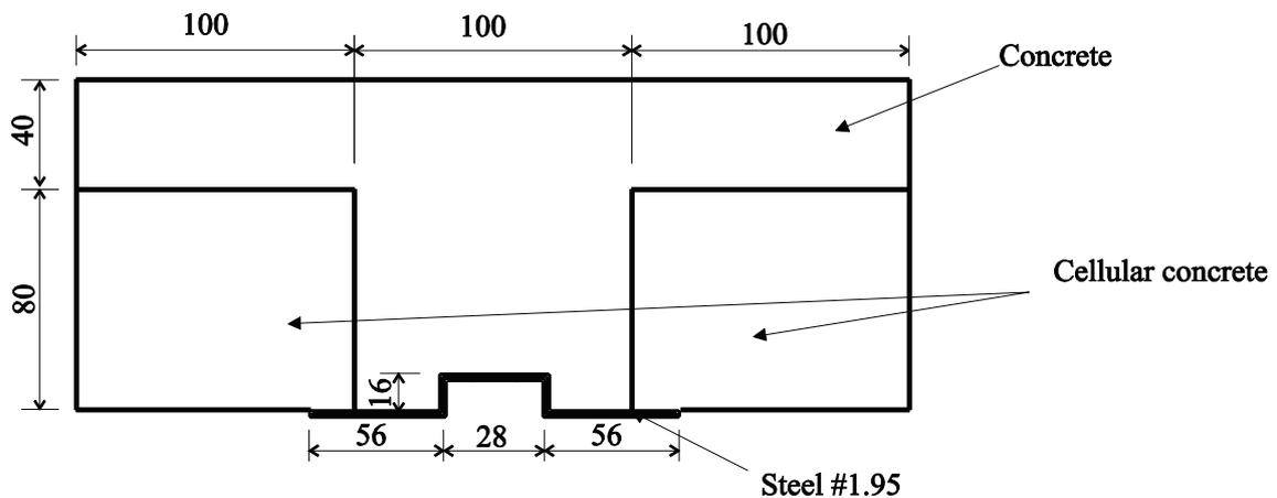
Figure 5 - Model with EPS/cement plate (dimensions in mm)
