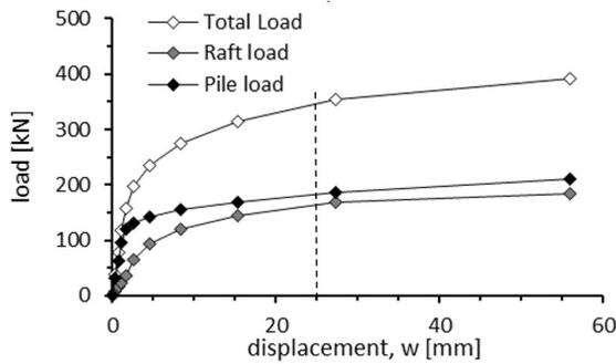
Figure 16. Load-settlement curve for case 9 - L=5m; t=0.1m
