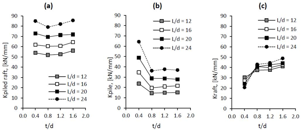
Figure 25. Effect of t/d ratio on piled raft, pile and raft responses
