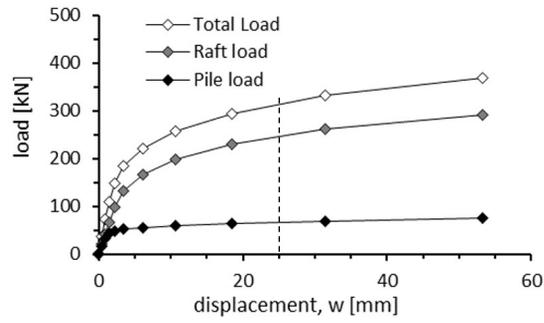
Figure 10. Load-settlement curves for case 3 -  $L=3m$ ;  $t=0.3m$
