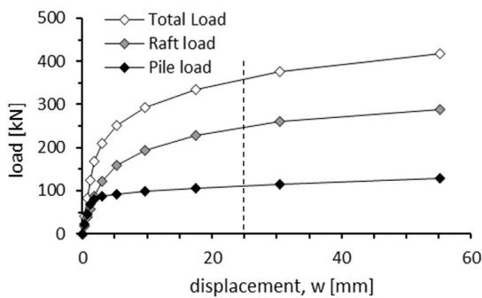
Figure 17. Load-settlement curves for case 10 - L=5m; t=0.2m
