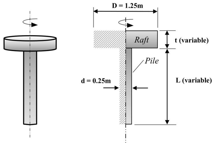
Figure 6. Geometry of the piled raft.
