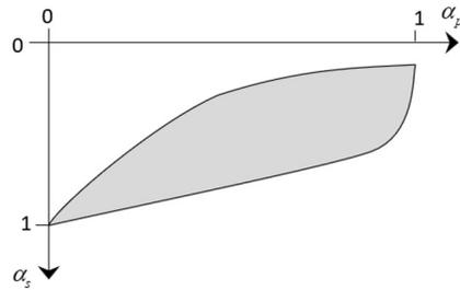
**Figure 1.** Correlation between settlement reduction coefficient,  $\alpha_s$ , and load sharing coefficient  $\alpha_{pr}$  of piled raft.
