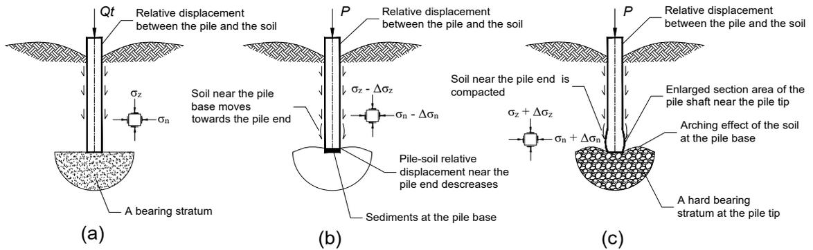
Figure 3. Stress state of soil element near pile end with different soil strengths at pile base (after Zhang et al. [26]).
