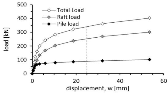
Figure 14. Load-settlement curves for case 7 - L=4m; t=0.3m
