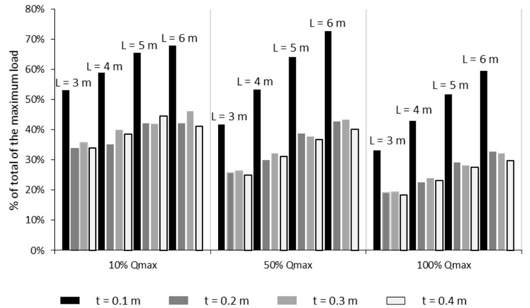
Figure 24. Portion of the maximum load taken by the total shaft resistance.
