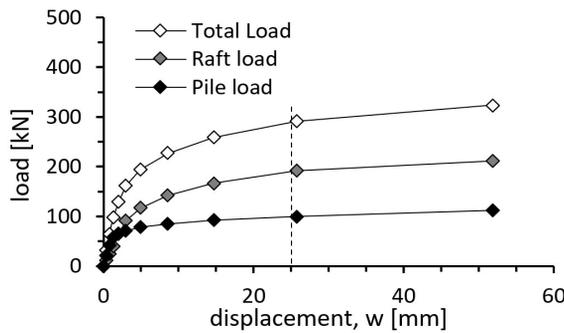
Figure 8. Load-settlement curve for case 1 - L=3m; t=0.1m
