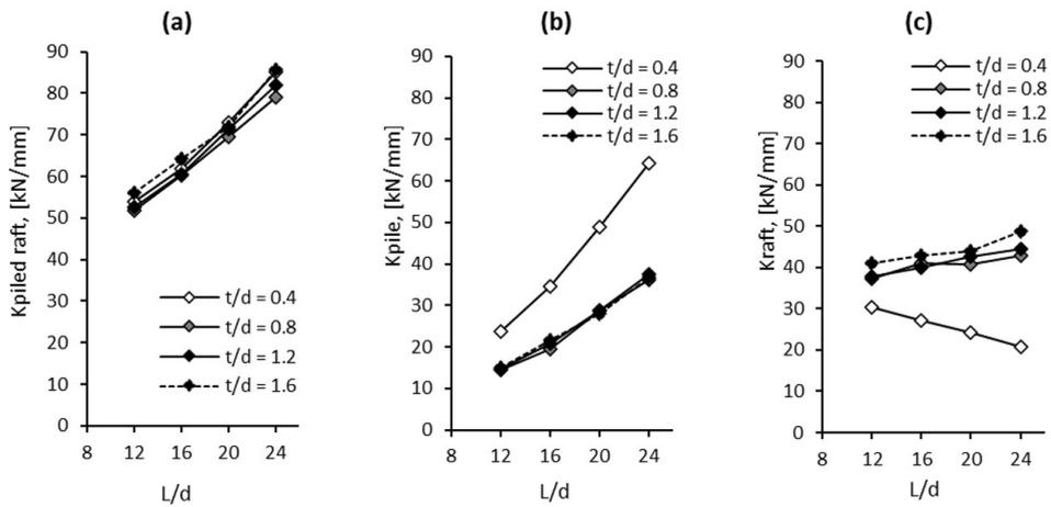
Figure 26. Effect of L/d ratio on piled raft, pile and raft responses.
