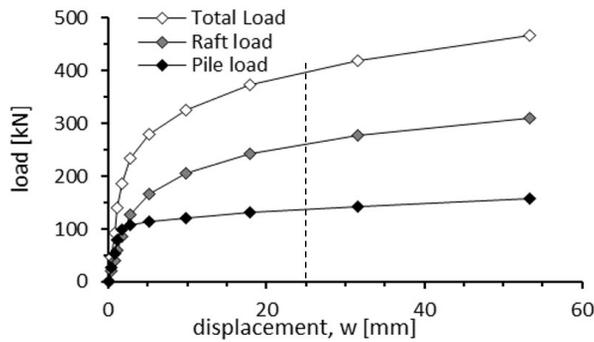
Figure 22. Load-settlement curves for case 15 - L=6m; t=0.3m
