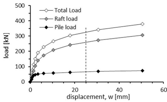
Figure 11. Load-settlement curves for case 4 -  $L=3m$ ;  $t=0.4m$
