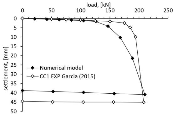
Figure 5. Load-settlement curves of the piled rafts by Garcia [9] versus numerical model.
