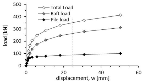
Figure 15. Load-settlement curves for case 8 - L=4m; t=0.4m
