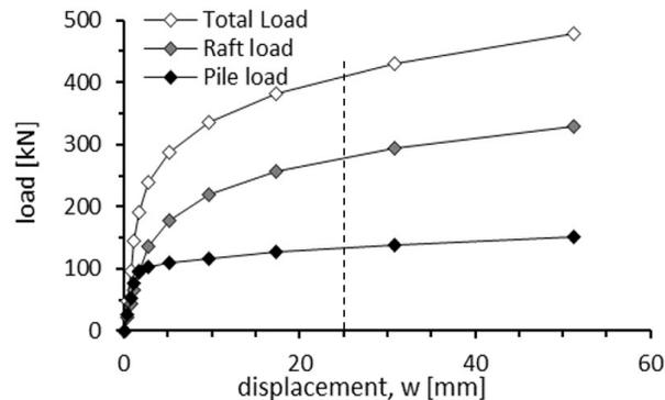
Figure 23. Load-settlement curves for case 16 - L=6m; t=0.4m
