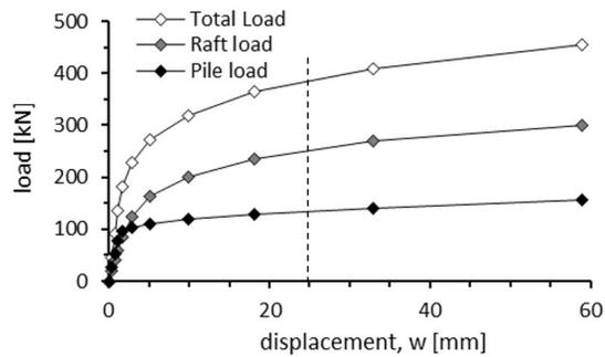
Figure 21. Load-settlement curves for case 14 - L=6m; t=0.2m
