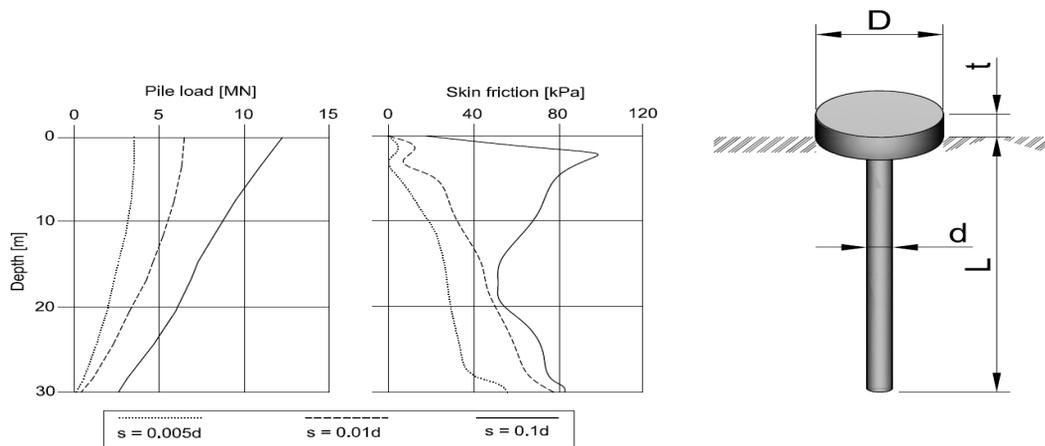
**Figure 2.** Influence of the pile-raft interaction on axial load transfer and skin friction with depth based on the Frankfurt Clay model (Katzenbach et al. [20]).
