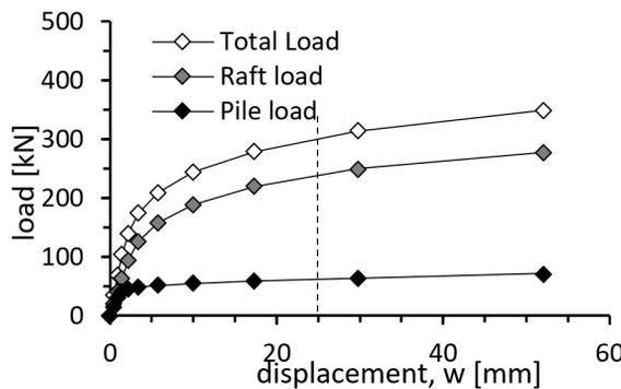
Figure 9. Load-settlement curves for case 2 - L=3m; t=0.2m
