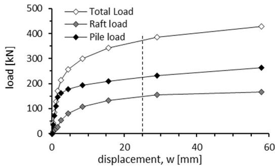
Figure 20. Load-settlement curves for case 13 - L=6m; t=0.1m
