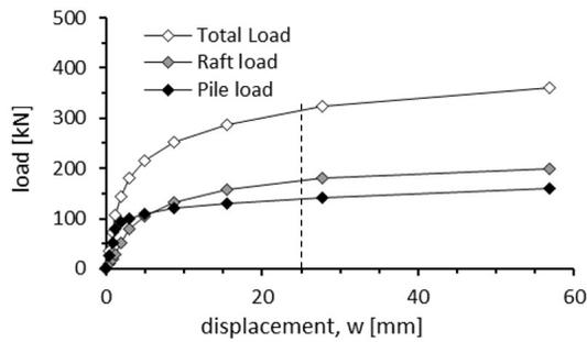
Figure 12. Load-settlement curves for case 8 -  $L=4m$ ;  $t=0.1m$
