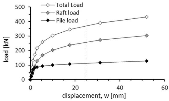
Figure 18. Load-settlement curves for case 11 - L=5m; t=0.3m
