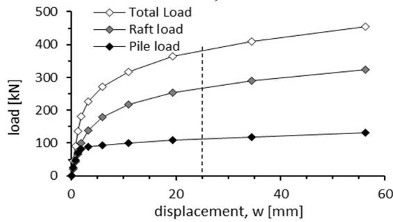
Figure 19. Load-settlement curves for case 12 - L=5m; t=0.4m
