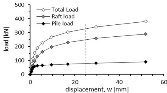
Figure 13. Load-settlement curves for case 6 -  $L=4m$ ;  $t=0.2m$
