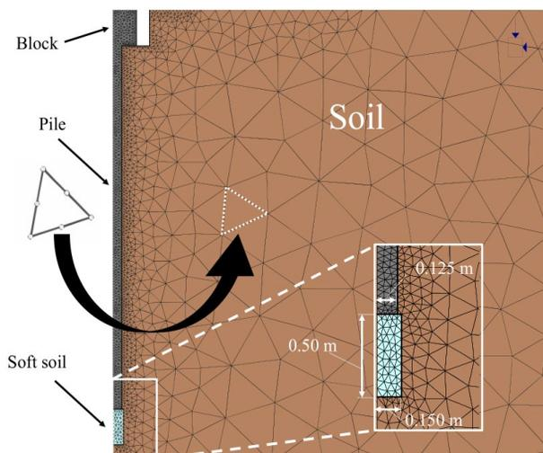
Figure 4. Numerical model for validation and detail of the soft material region inserted below the pile toe and graded mesh type and 6-noded triangle element.
