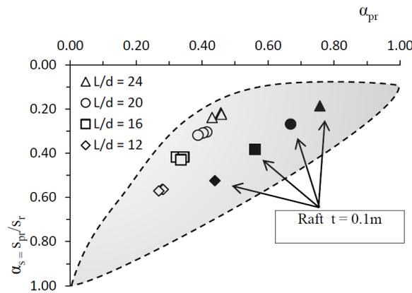
Figure 27. Evaluation of settlement reduction and load sharing for the piled rafts (at 50% of  $Q_{max}$ ).
