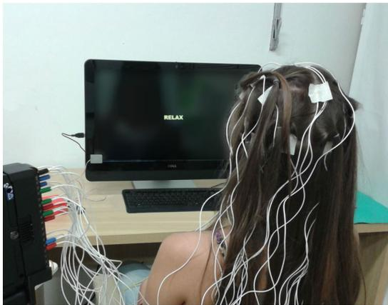
**Figure 2.** The experimental setup used for the VEP experiments. The volunteers sat comfortably in a chair while a set of images were presented on a computer screen placed at a distance of 70 cm. EEG data were collected throughout the experiment along with a synchronization signal used to indicate the presentation and valence of each image.
