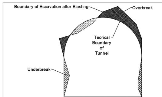
Figure 1 - Real and theoretical section of a tunnel.
