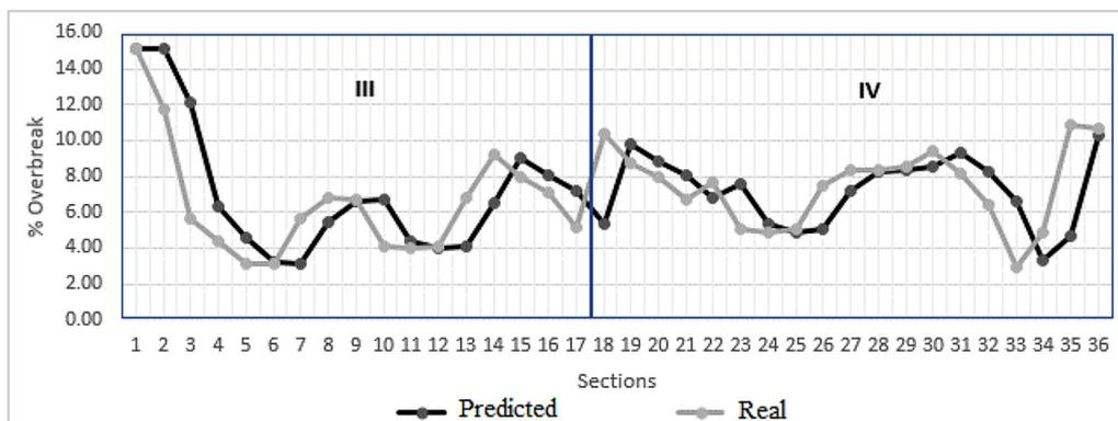
Figure 4 - Values of predicted and real % overbreak along the sections of the tunnel.
