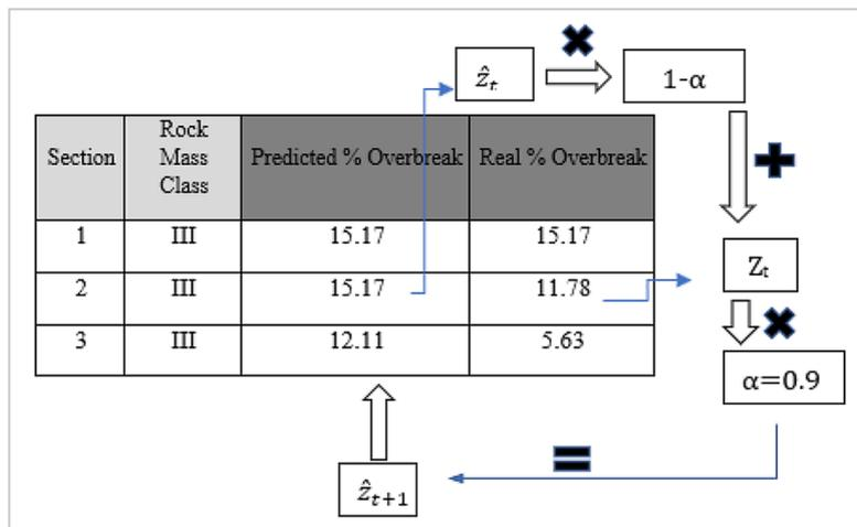
Figure 3 - Flowchart of applying of the model.
