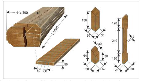
Figure 1 - Dimension of wood specimens and description of their extraction (Dimension in mm). Source: Morando et al. (2019).
