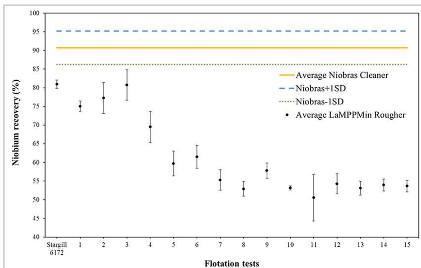
Figure 2 - Comparison between the niobium recovery average results in all flotation tests.
