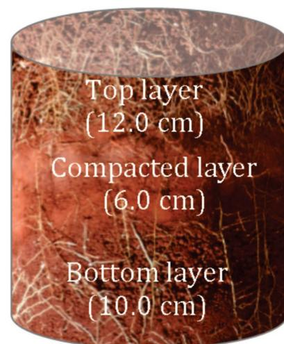
**Figure 1:** Schematic representation of the experimental pot, showing the top (layer A), compacted (layer B) and bottom layers (layer C) of the soil.
