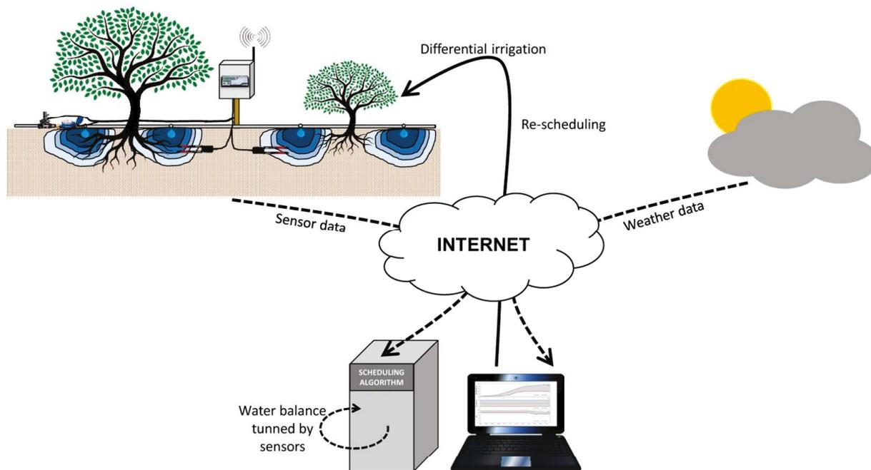
**Figure 2** - Organization chart for the operation of the semi-automatic irrigation management system (SOUZA; CONCHESQUI; SILVA, 2019)
