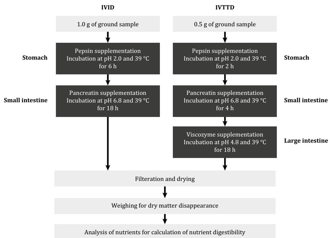
**Figure 1** - *In vitro* ileal disappearance (IVID) procedure and *in vitro* total tract disappearance (IVTTD) procedure (Boisen and Fernández, 1995; Boisen and Fernández, 1997; Recharla et al., 2019).
