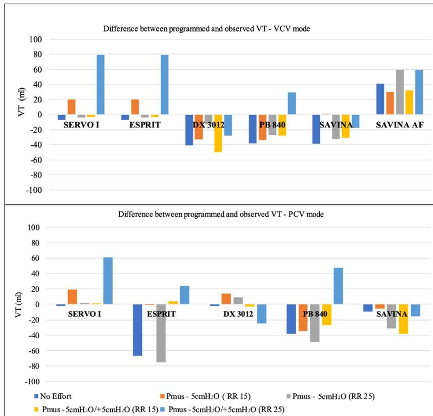
**Figure 3** - Difference between programmed and observed tidal volume in volume-controlled ventilation and pressure-controlled ventilation mode for the five ventilators in all simulated scenarios. The tidal volume programmed was 420mL.
