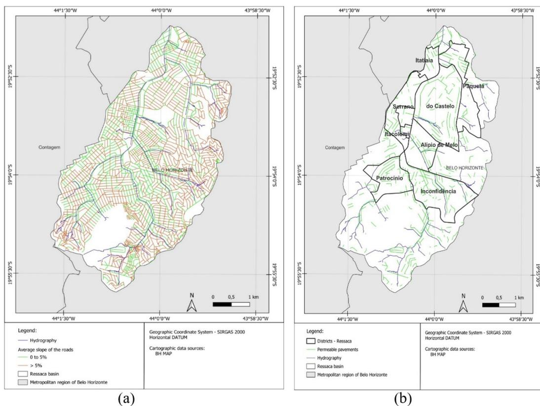
**Figure 7.** Maps indicating the slopes of the roads (a) and the areas selected for permeable pavement implementation, considering the districts with greater concentration of these areas (b).
