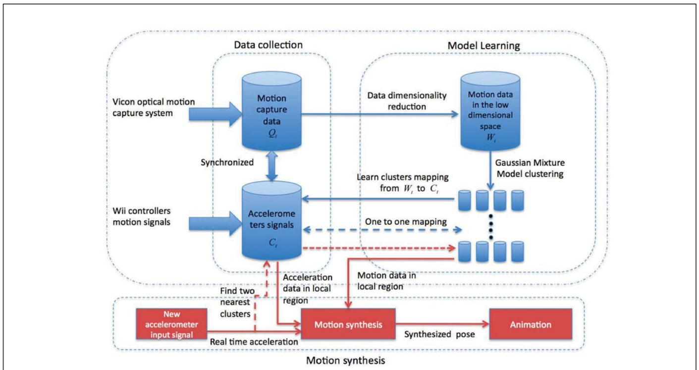
Figure 1. Motion estimation algorithm of the basketball motion model.
