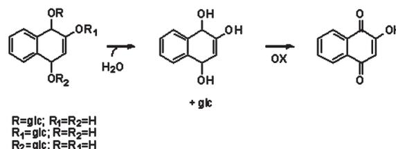
**Scheme 1.** Conversion of the three isomeric glucosides (hennosides) into the unique aglycone by hydrolysis in mildly acid conditions. Further transformation of the aglycone leads to the more stable lawsone by easy oxidation.
