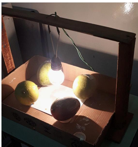
**Figure 1.** Picture of the apparatus used to evaluate the sunburn effect on mangoes.
