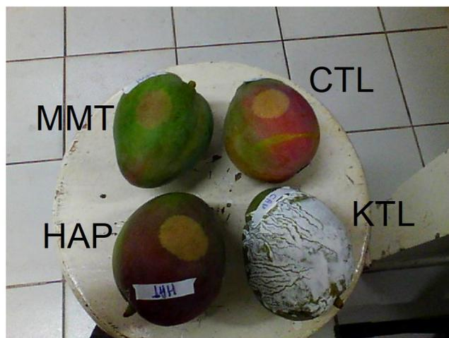
**Figure 3.** The general aspect of mangos coated with formulations based on kaolinite (KLT), hydroxyapatite (HAP), montmorillonite (MMT) and non-coated control (CTL), after 4 hours under incandescent radiation.
