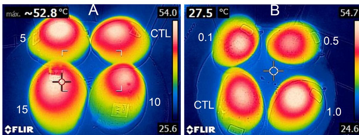
**Figure 4.** Thermography pictures of mangoes coated with photoprotective films based on galactomannan and hydroxyapatite at a) different galactomannan concentrations of 5.0, 10.0 and 15.0  $\text{mg mL}^{-1}$ , at fixed hydroxyapatite concentration of 0.1% (w/v) and b) different hydroxyapatite concentrations of 0.1, 0.5 and 1.0%, at fixed galactomannan concentration of 10  $\text{mg mL}^{-1}$ , submitted to 4 hours of incandescent radiation. ‘CTL’ stands for negative non-coated control.
