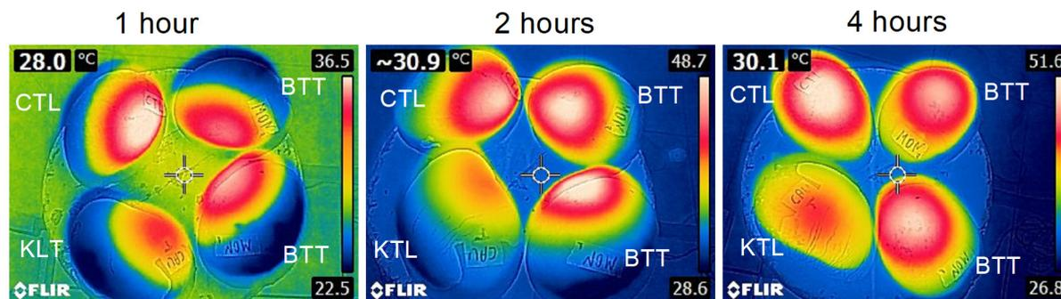
**Figure 5.** Thermography pictures of mangoes coated with photoprotective film based on galactomannan ( $5.0 \text{ mg mL}^{-1}$ ) and additive clays bentonite, BTT, ( $0.5\% \text{ w/v}$ ), submitted to different periods of incandescent radiation. 'CTL' stands for the negative control and the 'KLT' for the positive kaolinite control.
