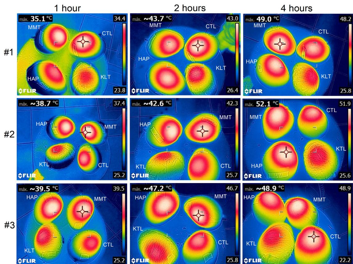
**Figure 2.** Thermography pictures results (triplicate) of mangoes coated with photoprotective film based on galactomannan at  $5.0 \text{ mg mL}^{-1}$  and additive clays (CTL: control, KLT: kaolinite, HAP: hydroxyapatite and MMT: montmorillonite) at 0.1%, submitted to different periods of incandescent radiation.
