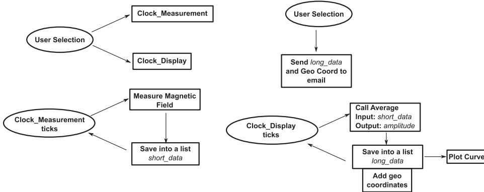
**Figure 2:** Deployed software application building blocks.
