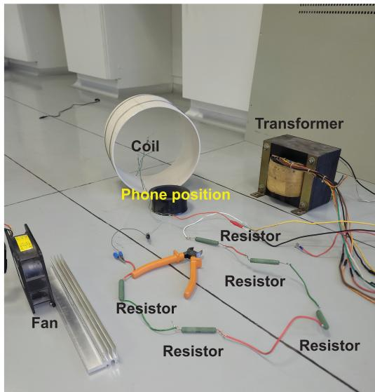
**Figure 9:** Setup to test the AC response of the mobile phone sensor. The plier at the center works as size reference.
