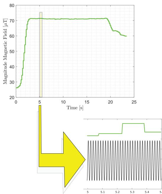
**Figure 10:** AC response of the coil. Inset shows a zoomed-in sector, alongside the expected oscillatory curve, not captured by the sensor.
