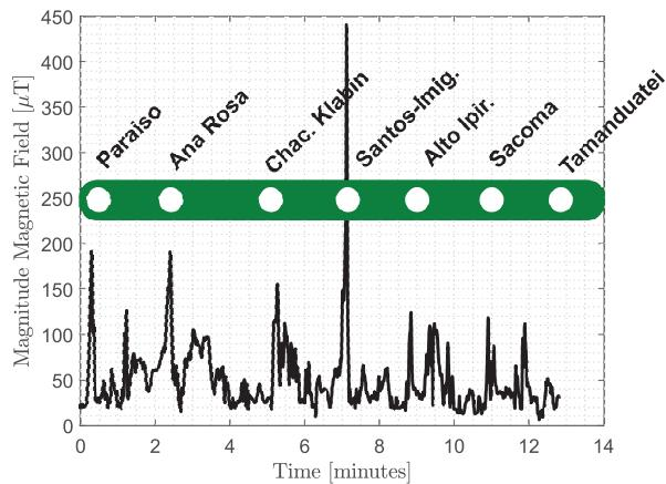
**Figure 7:** Measurements across São Paulo Line 2 (green) subway stations, names shown in the plot.
