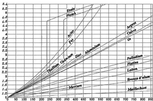
Figure 11 - Graphical behavior of resistance according to the Benoit's results. Credit: Ref. [35].
