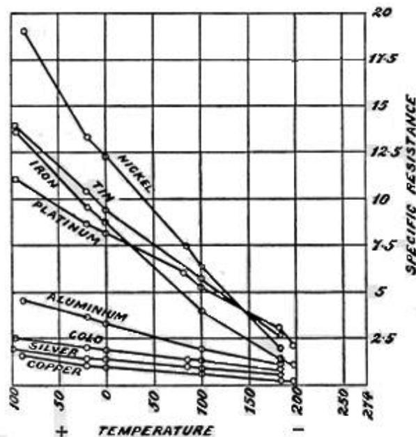
Figure 12 - Dewar's electrical conductivities of some metals at low temperatures. Credit: Ref. [38].
