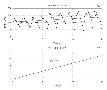
Figure 3. (a) Linear regression for the RMS parameter and (b) the respective index of fatigue (IF).
