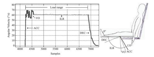
Figure 1. The angular velocity signal with the respective phases of the isokinetic knee extension exercise at 60°/s. Acceleration (ACC), velocity overshoot (VO), isokinetic load range (ILR) and deceleration (DEC).
