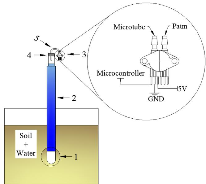
1 - Porous capsule; 2 - PVC tube; 3 - Pressure sensor MPX5100dp; 4 - Sealing rubber; 5 - Microtube; Patm - Atmospheric pressure; GND - Ground
