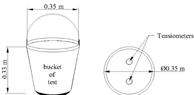
Figure 3. Arrangement of tensiometers
