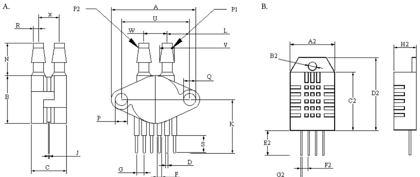
Dimensions in mm: (A) A - 29.85, B - 18.16, C - 11.05, D - 0.84, F - 1.63, G - 2.54, J - 0.41, K - 18.42, L - 7.62, N - 11.18, P - Ø4.04, Q - Ø4.04, R - 2.11, S - 6.10, U - 23.11, V - 4.93, W - 8.38, and X - 7.06; (B) A2 - 15.10, B2 - Ø3.00, C2 - 20.00, D2 - 25.10, E2 - 8.50, F2 - 2.00, G2 - 0.50, and H2 - 7.70
